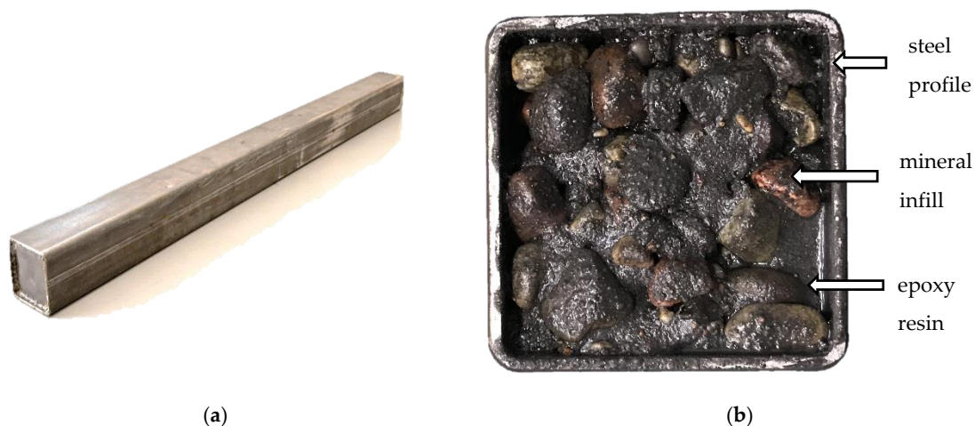
Figure 1. Steel-polymer concrete beam (a) general view; (b) cross-section view.
