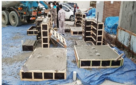
**Figure 2.** Application test of early strength concrete in the Batcher plant.
