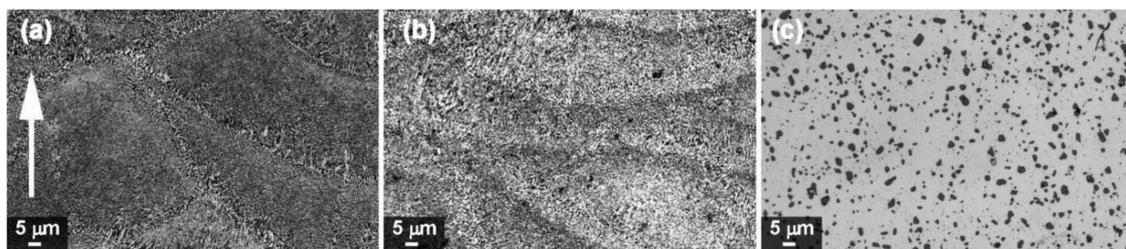
**Figure 4.** Optical images of A357 samples: (a) as-built; (b) after stress-relieving; (c) after  $\text{T6}_{B,170,3}$  heat treatment. The white arrow indicates building direction.
