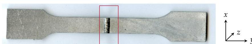
**Figure 1.** Welded tensile test specimen, area of XCT testing highlighted in red.
