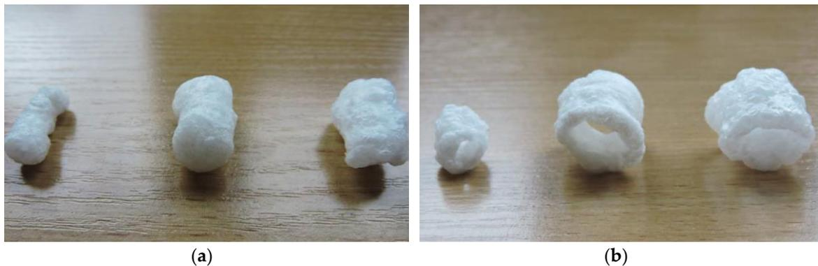
**Figure 1.** Obtained starch-based foams: (a) circular die and (b) ring die.
