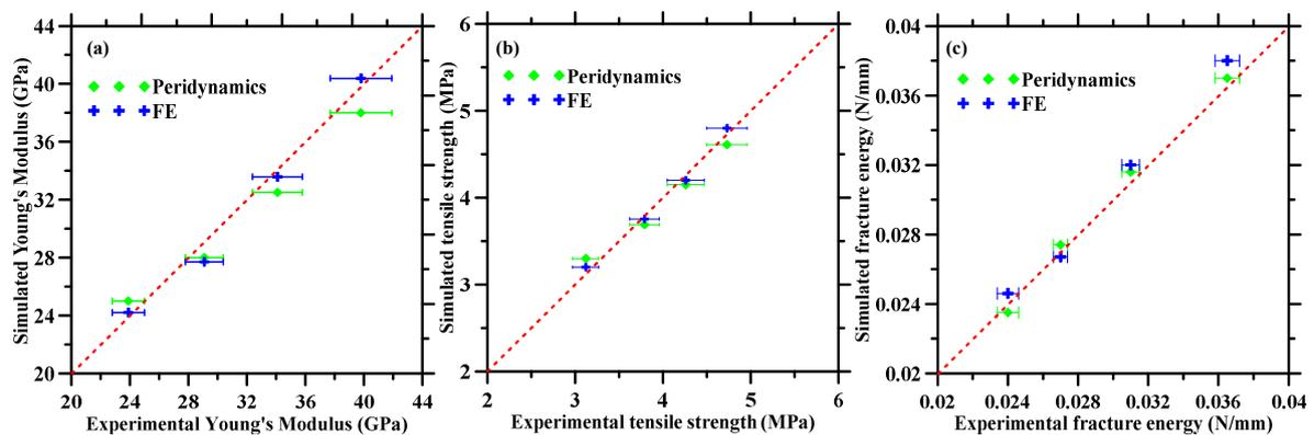
**Figure 9.** Correlation between experimental and simulated (peridynamics and finite element (FE) approach) (a) Young's modulus and (b) tensile strengths and (c) fracture energy of mortars with various dosage of waste iron powder.
