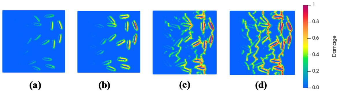
**Figure 5.** Progressive damage observed in iron powder (10%) modified HCP corresponding to applied tensile strains of (a)  $24 \mu\epsilon$ , (b)  $78 \mu\epsilon$ , (c)  $121 \mu\epsilon$  and (d)  $130 \mu\epsilon$ .
