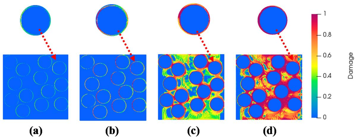
**Figure 7.** Progressive damage (interface/matrix) observed in iron powder (10%) modified mortar corresponding to applied tensile strains of (a)  $52 \mu\epsilon$ , (b)  $105 \mu\epsilon$ , (c)  $153 \mu\epsilon$  and (d)  $208 \mu\epsilon$  (the interface damage is highlighted in zoomed pictures).
