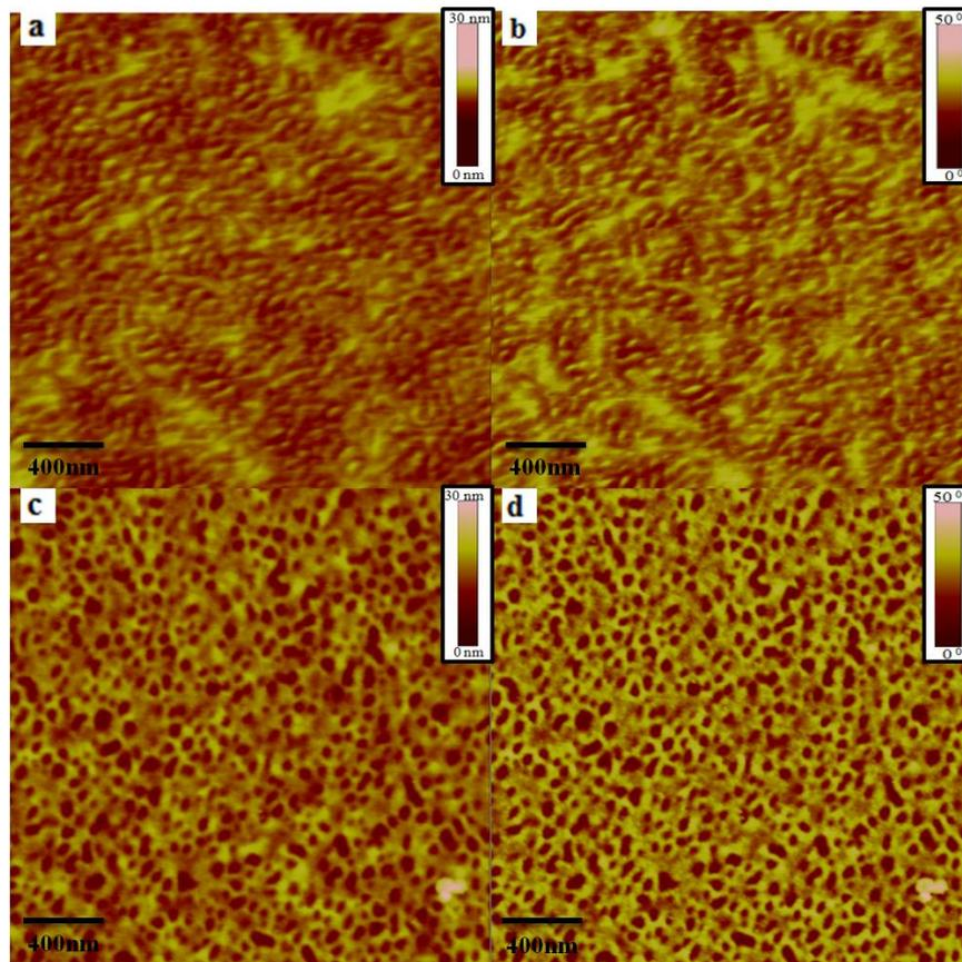
**Figure 4.** TP-AFM height (left) and phase (right) images for the neat samples of PS<sub>25</sub>-b-PB<sub>23</sub>-b-PI<sub>12</sub> (a,b) and PS<sub>45</sub>-b-PB<sub>34</sub>-b-PI<sub>74</sub> (c,d) respectively after 24 hours annealing in benzene vapors inside the autoclave chamber (solvent vapor annealing).
