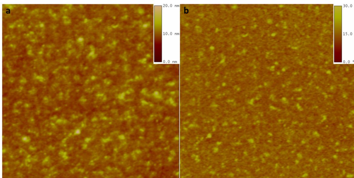
**Figure 8.** TP-AFM height (a) and phase (b) images for PS40-b-PB40\_PS- $\gamma$ -Fe<sub>2</sub>O<sub>3</sub> composite thin film with loading rate 12.5% wt after 24h SVA.
