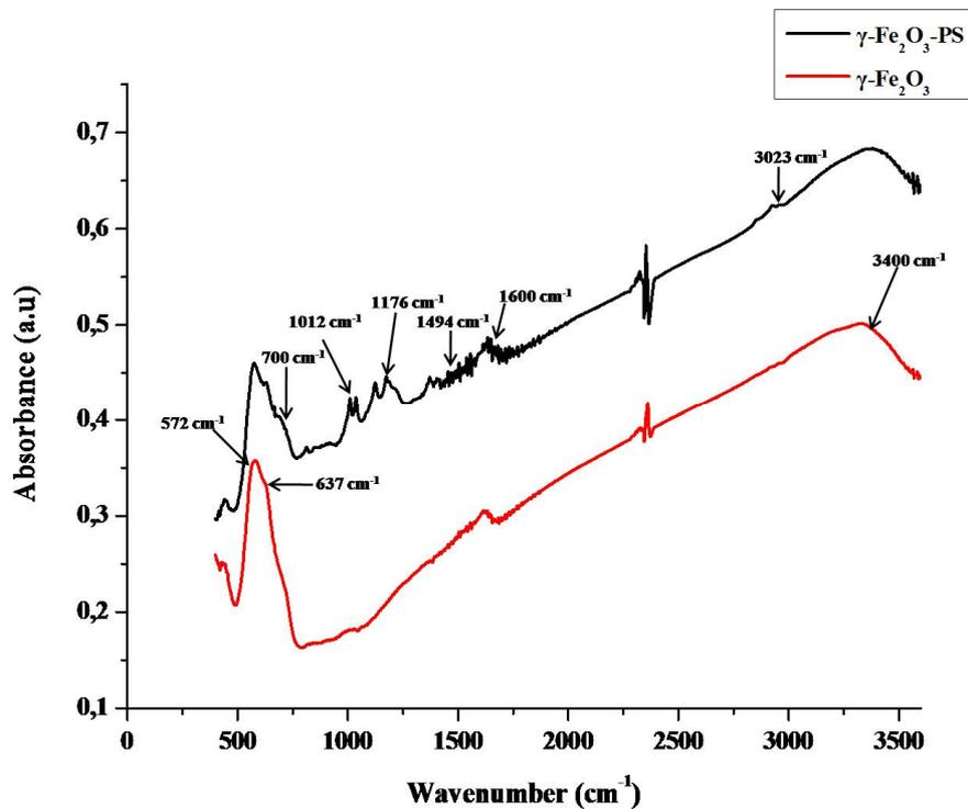
**Figure 1.** Infrared spectra of  $\gamma\text{-Fe}_2\text{O}_3$  magnetic nanoparticles (indicated with red) and  $\gamma\text{-Fe}_2\text{O}_3$  magnetic nanoparticles functionalized with polystyrene chains (indicated with black).
