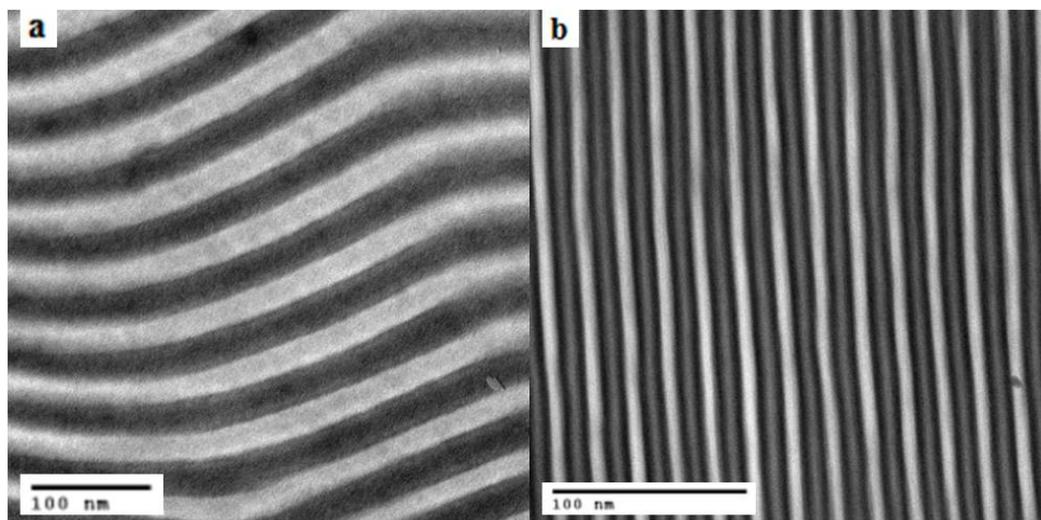
**Figure 5.** TEM images for the two linear triblock terpolymers of different total molecular weight indicating the PS-b-PB-b-PI<sub>3,4</sub> sequence. Image (a) corresponds to PS<sub>45</sub>-b-PB<sub>34</sub>-b-PI<sub>74</sub> and image (b) to PS<sub>25</sub>-b-PB<sub>23</sub>-b-PI<sub>12</sub> respectively. The indices next to the blocks in both samples indicate the number average molecular weight of each block respectively.
