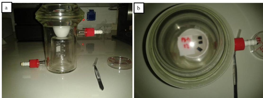
**Figure 7.** Side (a) and top (b) view of the improvised apparatus for the solvent vapor annealing procedure. Within this autoclave chamber, a glass substrate is evident up on which the Si wafers are deposited beneath which the solvent resides which stands on top of solvent deposit in a specific smaller chamber.
