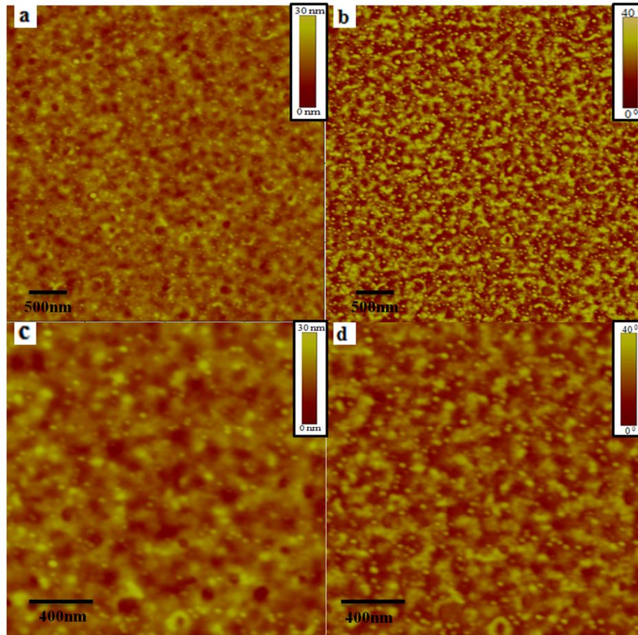
**Figure 6.** TP-AFM height (a,c) and phase (b,d) images for as-spun PS<sub>40</sub>-b-PB<sub>40</sub>-PS- $\gamma$ -Fe<sub>2</sub>O<sub>3</sub> composite thin film. Two different scan size of 4  $\mu$ m x 4  $\mu$ m & 2  $\mu$ m x 2  $\mu$ m(enlarged) views depict the NPs arrangement with loading rate 10% wt.
