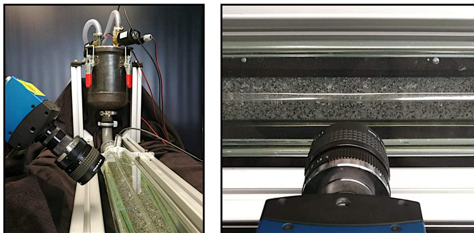
**Figure 2.** Camera setup (left) and close up of the model-fluid (right). The black cloths are used to reduce scattering.
