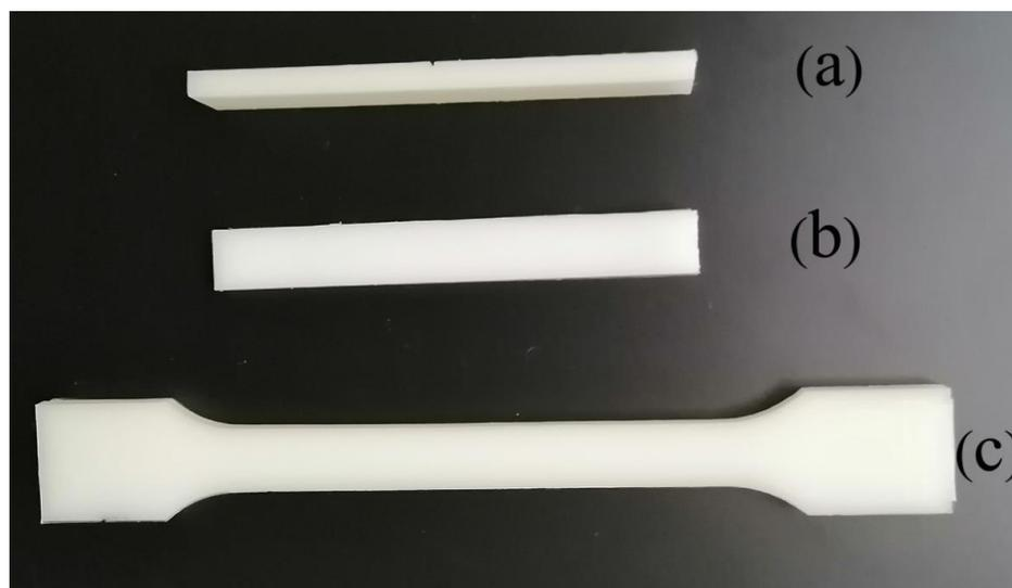
**Figure 1.** (a) Notched Charpy impact test specimen, (b) flexural test specimen, and (c) tensile test specimen.
