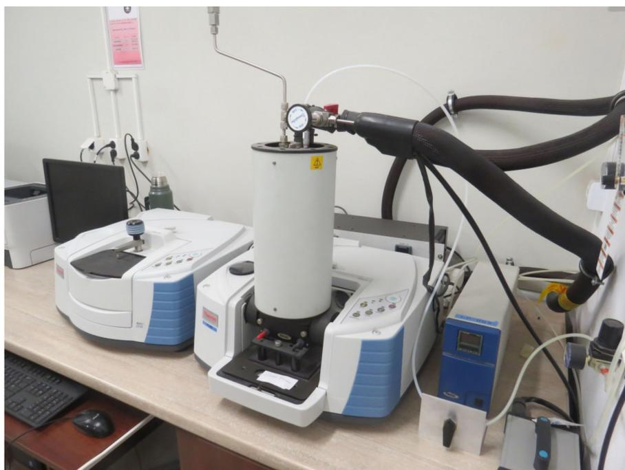
**Figure 3.** FTIR spectrometer at the accredited ITB Fire Laboratory in Pionki, Poland.
