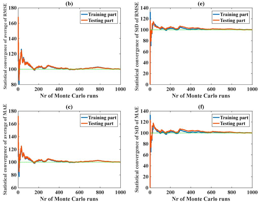
**Figure 3.** Convergence of random sampling in the case of using C-ANN-[3–20–20–1] for the average values of (a)  $R^2$ , (b) RMSE, and (c) MAE; for the standard deviation (SD) values of (d)  $R^2$ , (e) RMSE, and (f) MAE.
