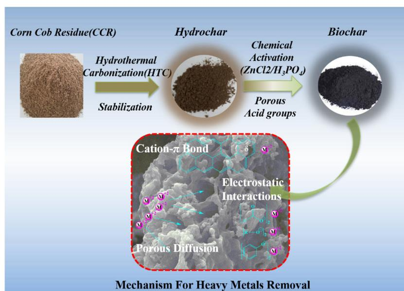
**Figure 2.** Concept of Biochars preparation and their applications for heavy metal ion removal through adsorption mechanisms.
