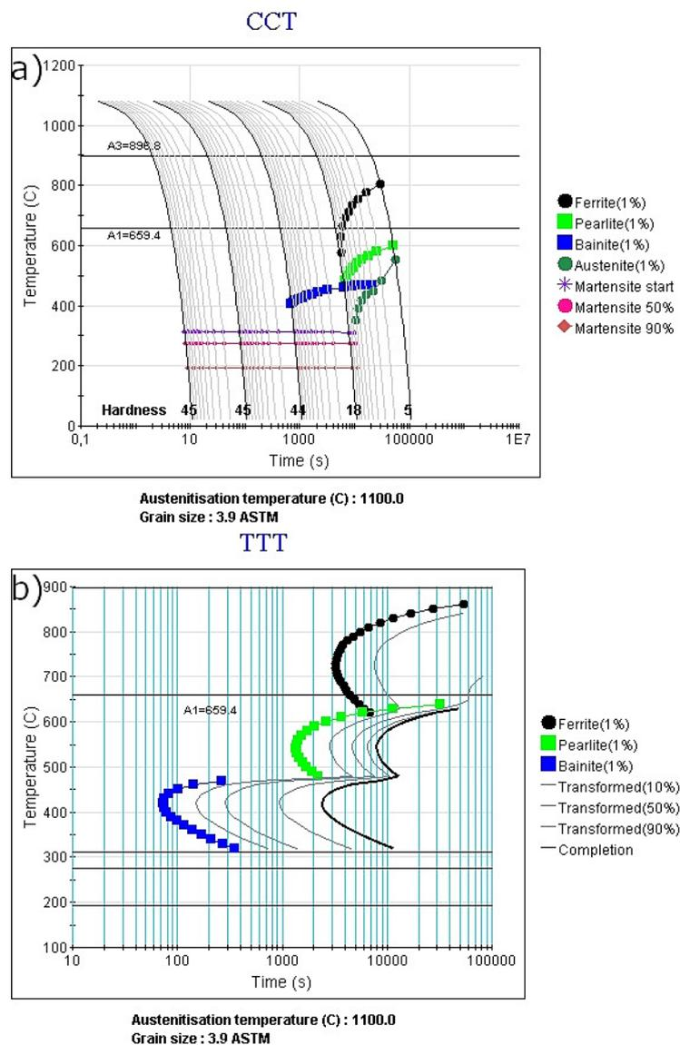
**Figure 3.** Non-equilibrium diagrams for analyzed steel: (a) CCT diagram; (b) TTT diagram.
