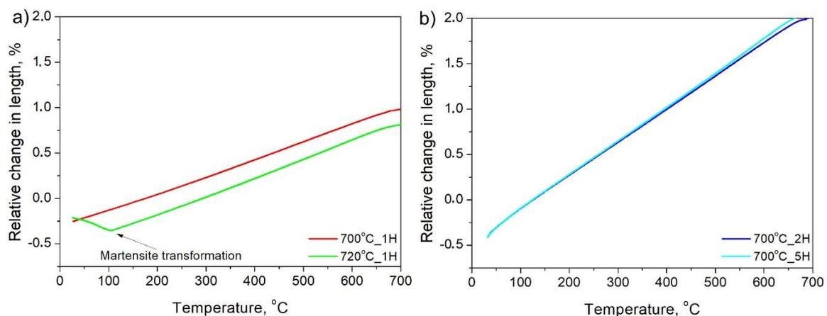
**Figure 7.** Dilatometric results during cooling to room temperature after intercritical annealing: (a) annealing at 700 and 720 °C for 1 h; (b) annealing at 700 °C for 2 and 5 h.
