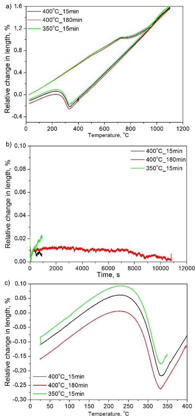
**Figure 4.** Dilatometric curves of steel during isothermal bainitic transformation: (a) full curves; (b) during isothermal holding; (c) during cooling to room temperature.
