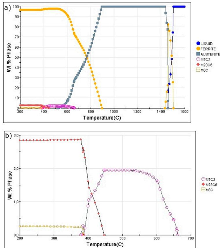
**Figure 2.** Phase evolution diagram of the steel in equilibrium conditions: (a) full diagram; (b) left bottom magnified part of the diagram.
