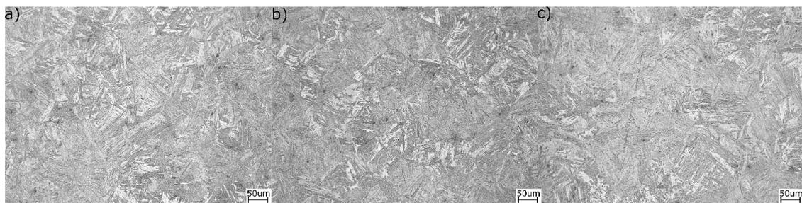
**Figure 5.** Microstructure of steel after isothermal holding in bainite region: (a) 400 °C, 15 min; (b) 400 °C, 180 min; (c) 350 °C, 15 min.
