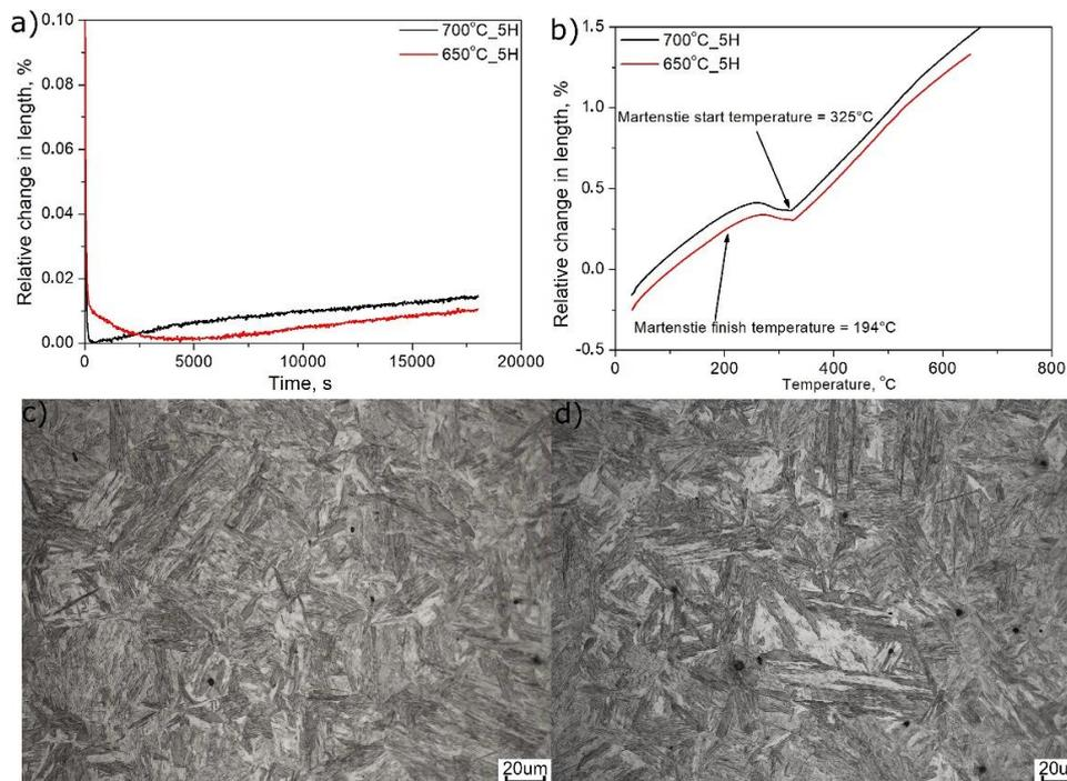
**Figure 6.** Results of dilatometry and microstructure investigation of simulated coiling process: (a) isothermal step; (b) cooling to room temperature; (c) microstructure after cooling from 700 °C; (d) microstructure after cooling from 650 °C.
