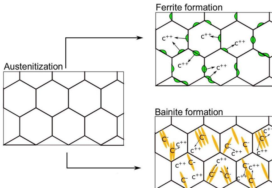
**Figure 10.** Schematic representation of carbon enrichment of the austenite during coiling and bainite transformation.
