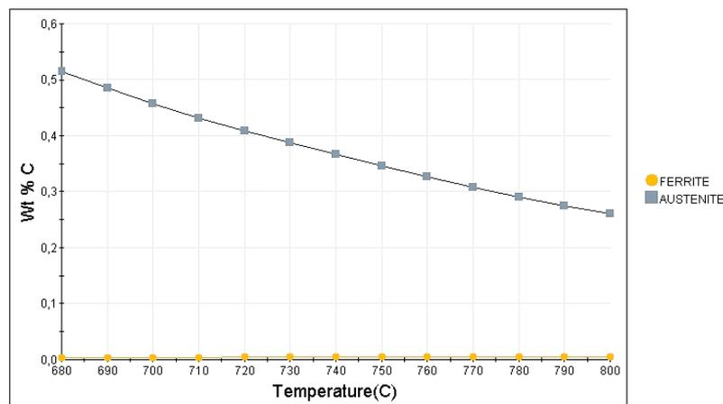
**Figure 13.** JMatPro simulation of carbon enrichment in the austenite at different intercritical temperatures.
