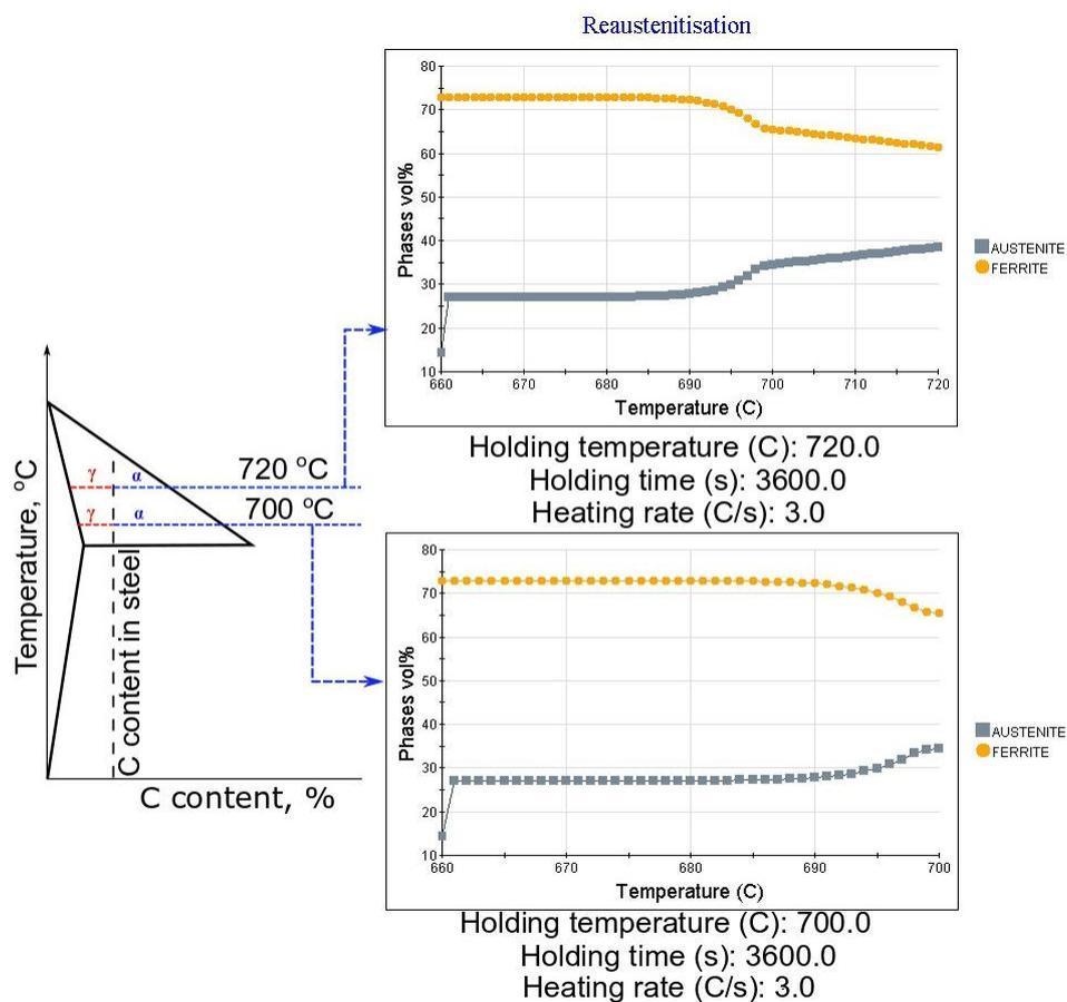
**Figure 12.** Schematic representation of a lever rule and theoretical calculations using JMatPro for intercritically annealed steels at 720 and 700 °C.
