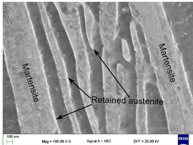
**Figure 9.** SEM micrograph of the sample intercritically annealed at 720 °C showing the retained austenite and martensite morphologies.
