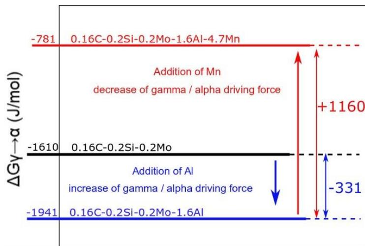
**Figure 11.** Theoretical calculations of Al and Mn effects on a driving force at 400 °C [15].
