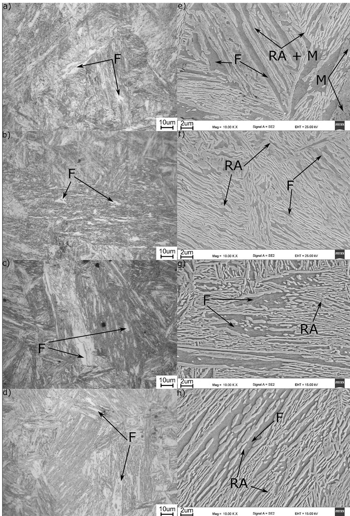
**Figure 8.** Light and scanning electron microscopy microstructures of intercritically annealed steel (a–e) 720 °C, (b–f) 700 °C, 1 h, (c–g) 700 °C, 2 h, (d–h) 700 °C, 5 h. F—ferrite, M—martensite, RA—retained austenite.
