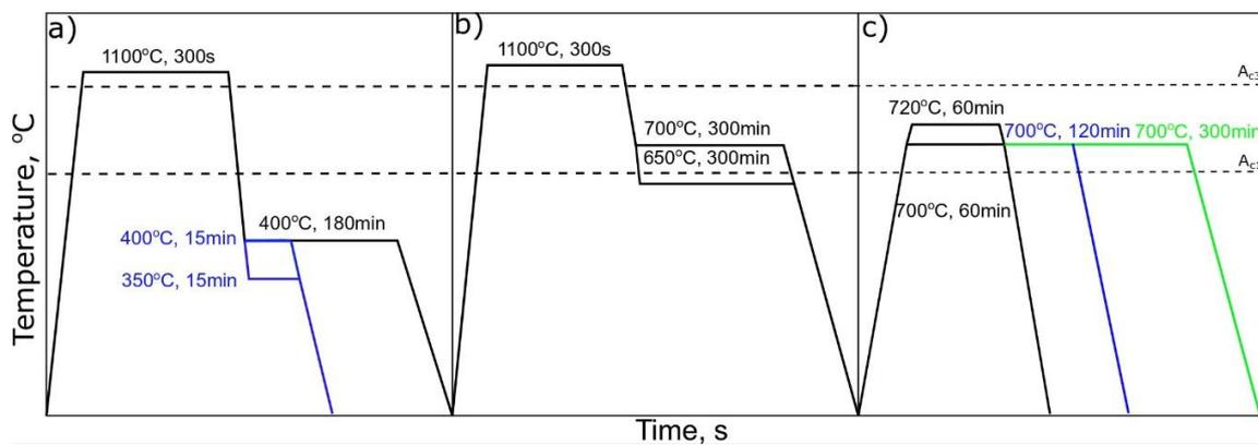
**Figure 1.** Different heat treatment schedules for analyzed steel: (a) in bainite region; (b) coiling simulation (ferrite region); (c) intercritical annealing.
