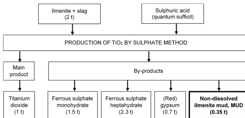
**Figure 1.** By-products generated per ton of the final product during the production of TiO<sub>2</sub> using the sulphate method (data calculated according to a Spanish factory in Huelva [11–13]).
