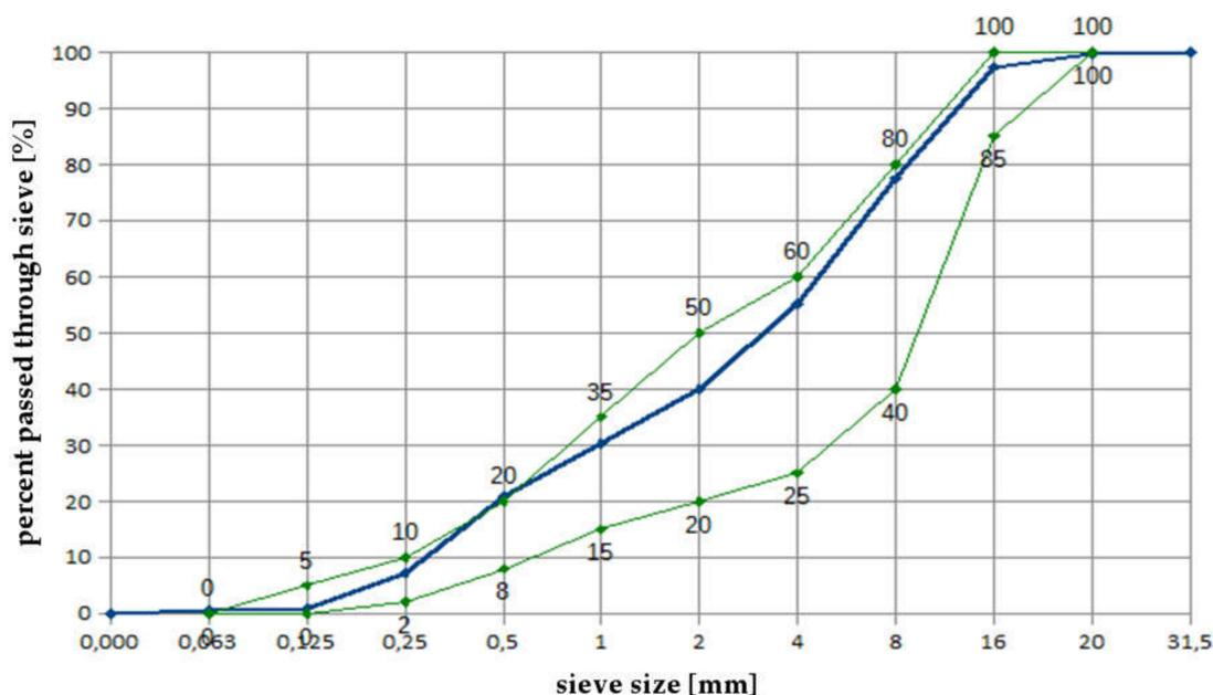
Figure 3. Sieving curves of aggregate mix used for concretes.
