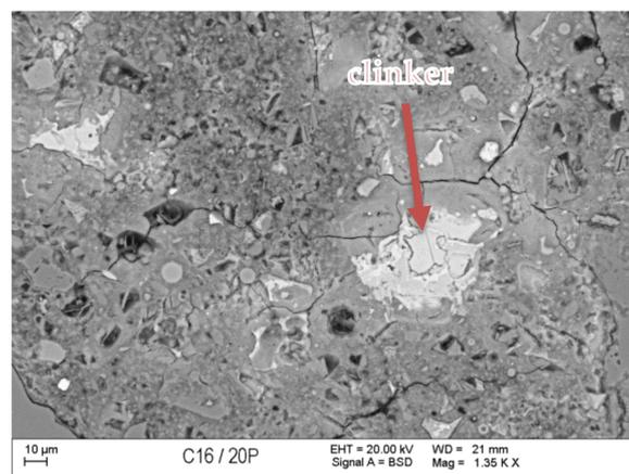
Figure 12. BSE image of FA concrete sample.
