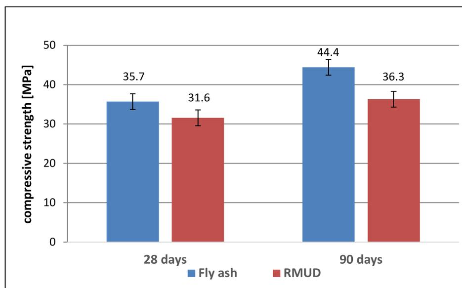
**Figure 5.** Compressive strength of concretes.
