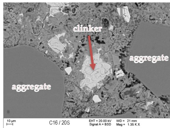
Figure 13. BSE image of RMUD concrete sample.
