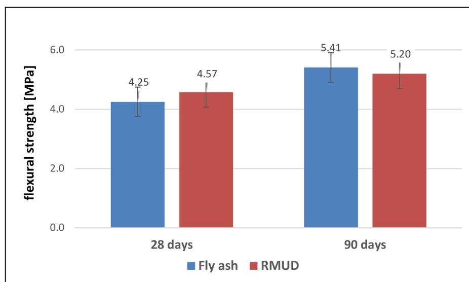
Figure 6. Flexural strength of concretes.
