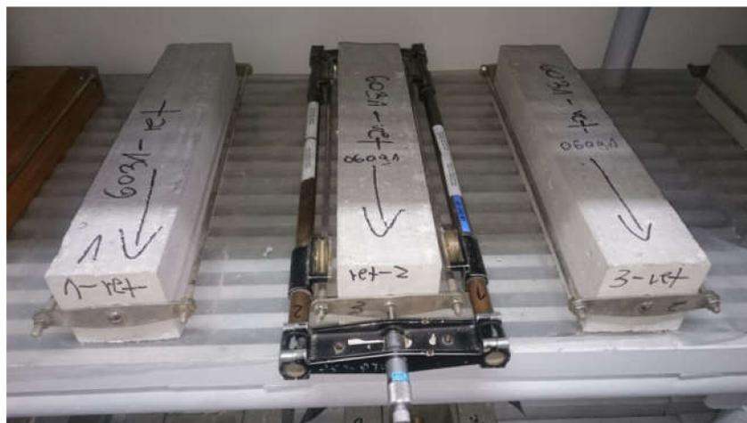
**Figure 4.** Measure of sample during shrinkage test.
