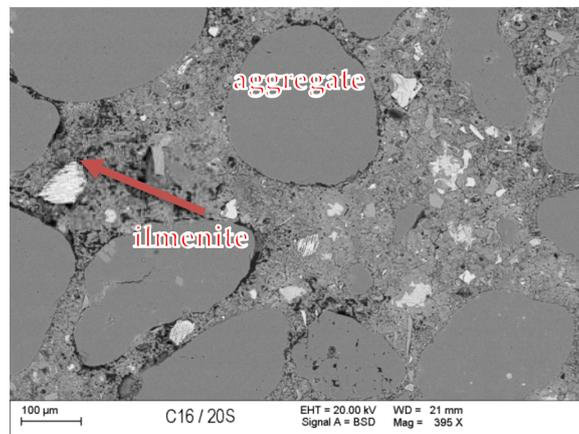
Figure 11. BSE image of RMUD concrete sample.
