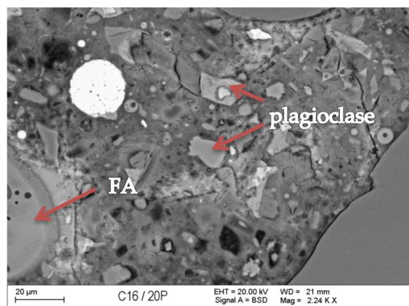
Figure 14. BSE image of FA concrete sample.
