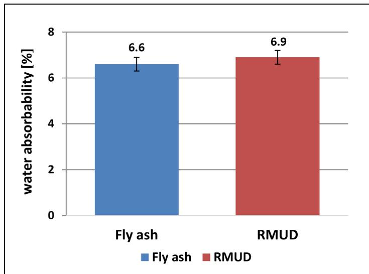
Figure 7. Water absorbability of concrete.
