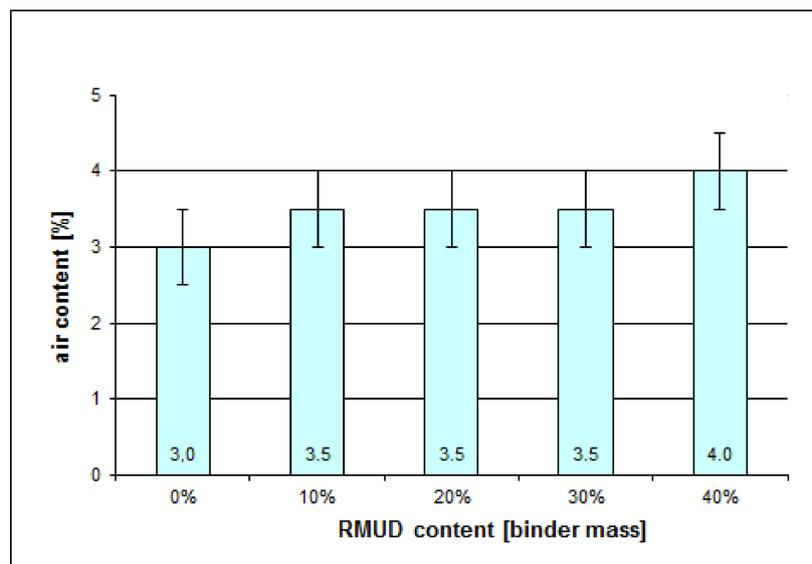
**Figure A1.** Influence of addition RMUD on air content in mortar.
