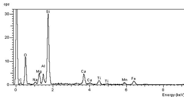
**Figure 16.** EDS spectrum of silicon dioxide glass phase.
