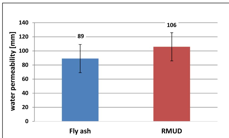
Figure 8. Average values of water permeability through concrete.
