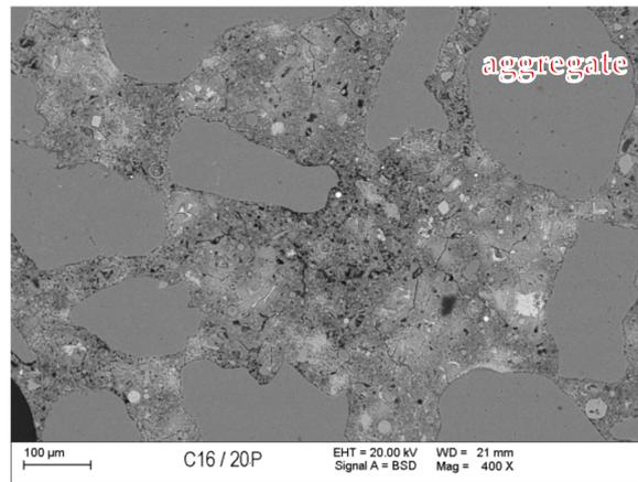
Figure 10. Back-scattered electrons (BSE) image of concrete with fly ash (FA).
