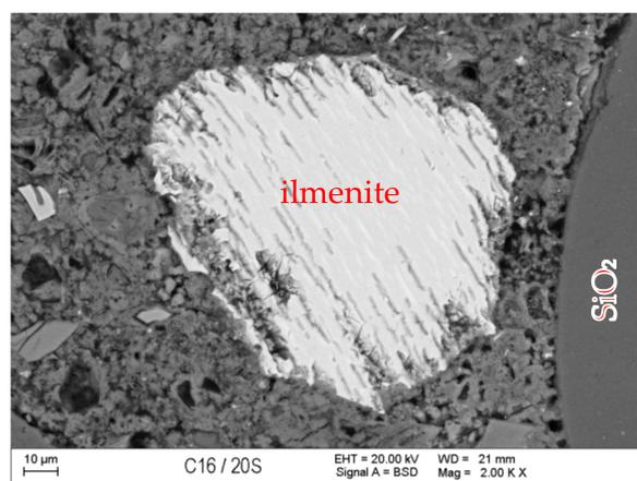
Figure 15. BSE image of RMUD concrete sample.
