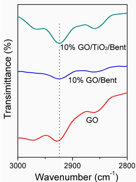
**Figure S1.** FTIR spectra of GO, 10% GO/Bent and 10% GO/TiO<sub>2</sub>/Bent sponges.
