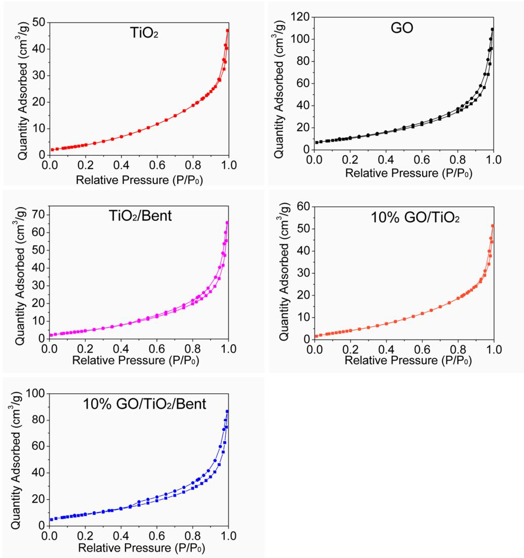
**Figure S3.** The  $\text{N}_2$  adsorption-desorption isotherms of  $\text{TiO}_2$ ,  $\text{GO}$ ,  $\text{TiO}_2/\text{Bent}$ ,  $10\%$   $\text{GO}/\text{TiO}_2$  and  $10\%$   $\text{GO}/\text{TiO}_2/\text{Bent}$ .
