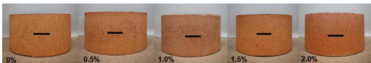
Figure 14. Efflorescence on bricks for mixes with 0%, 0.5%, 1.0%, 1.5%, and 2.0% CBs.
