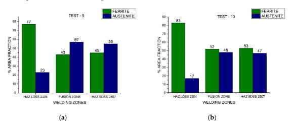
Figure 12. Area fraction through the distinct welded zones to 130 A: (a) Test #9 and (b) Test #10.
