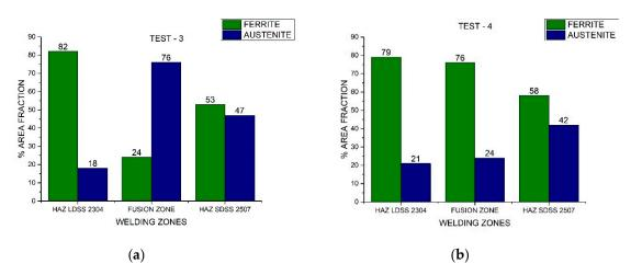
Figure 8. Area fraction through the distinct welded zones: (a) Test #3 and (b) Test #4.
