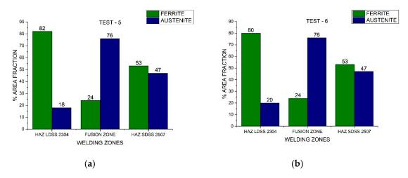
Figure 10. Area fraction through the distinct welded zones to 220 A: (a) Test #5 and (b) Test #6.
