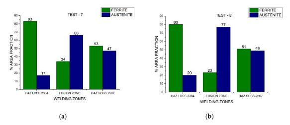
Figure 11. Area fraction through the distinct welded zones to 175 A: (a) Test #7 and (b) Test #8.
