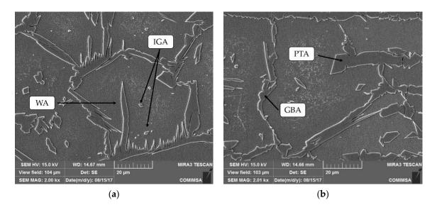
**Figure 9.** SEM micrographs of the heat-affected zone: (**a**) lean duplex stainless steel (LDSS) 2304; and (**b**) SDSS 2507. WA: Widmanstätten austenite; IGA: intragranular austenite; PTA: partially transformed austenite; GBA: grain boundary austenite.
