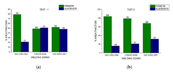
Figure 7. Area fraction through the distinct welded zones: (a) Test #1 and (b) Test #2.
