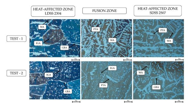
**Figure 5.** Welded zones by optical microscope to  $50 \times : 130$  A welding current.
