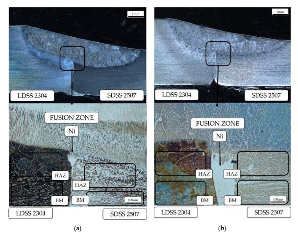
Figure 4. Welded zones by optical microscope to 10 ×: (a) Test #3 and (b) Test #1.
