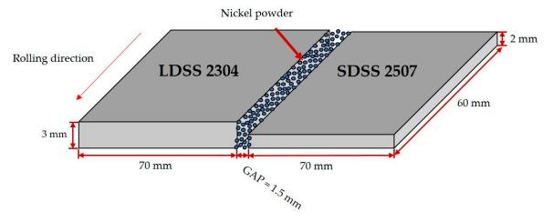
Figure 1. Scheme of the dissimilar duplex stainless-steel butt joint.
