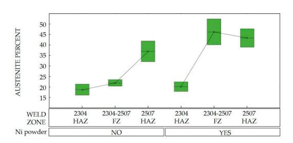
Figure 2. Box plot for austenite percentage. FZ: fusion zone; HAZ: heat-affected zone.
