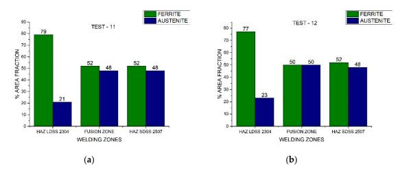
Figure 13. Area fraction through the distinct welded zones: (a) Test #11 and (b) Test #12.
