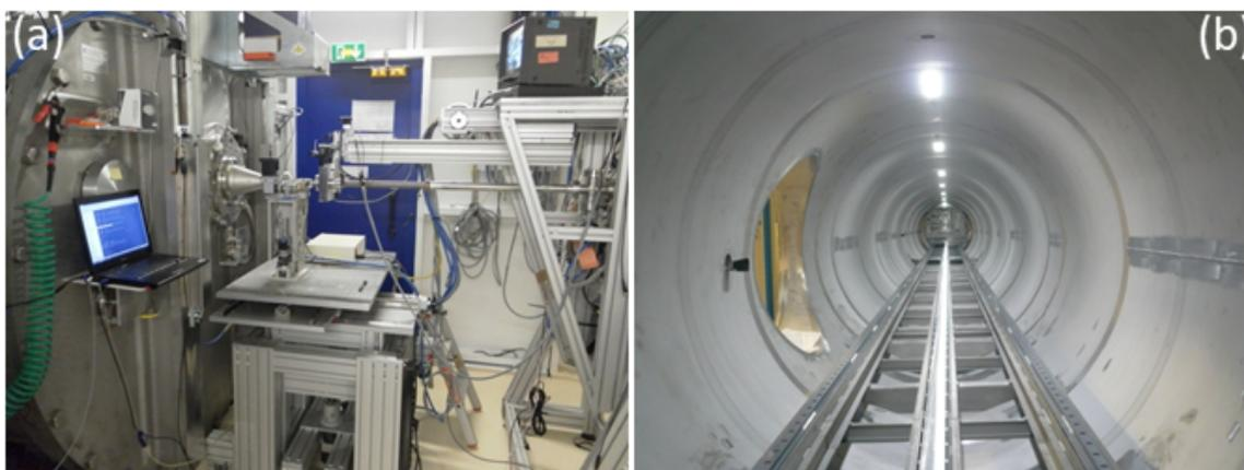
**Figure 4.** Experiment station at ID02 beamline at the ESRF. (a) The photo displays the sample table and stages, incident side telescopic tube, and the entrance cone of the detector tube. (b) Inside view of the 34 m long and 2 m diameter detector tube showing the detector carriage at the end.
