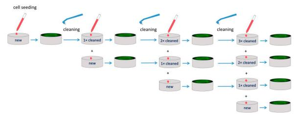
Figure 1. Scheme of the experiment: cell seeding on new as well as repeatedly cleaned titanium samples.
