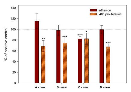
**Figure 3.** Comparison of cell adhesion and proliferation on the surface of new titanium samples assessed by CCK-8 assay in four independent experiments. The standard errors were calculated from five replicates. Data expressed as a percentage of positive control. Error bars indicate means  $\pm$  standard deviations. Asterisks above the bars indicate significant differences (\* p < 0.05, \*\* p < 0.01, \*\*\* p < 0.001) between titanium samples and positive controls.
