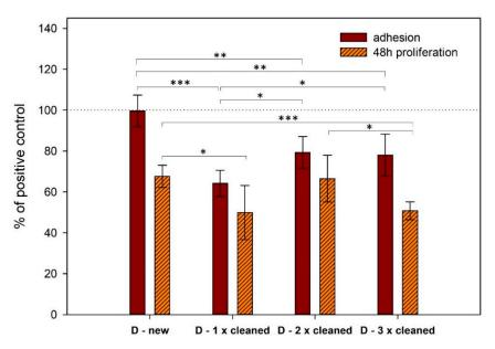
**Figure 4.** Comparison of cell adhesion and proliferation on the surface of new and different times cleaned same titanium samples assessed by CCK-8 assay. The standard errors were calculated from five replicates. Data expressed as a percentage of positive control. Error bars indicate means  $\pm$  standard deviations. Asterisks represent statistical significance between respective groups (\* p < 0.05, \*\* p < 0.01, \*\*\* p < 0.001).
