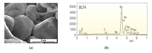
Figure 2. SEM images of fractures (a) and EDS emission spectrum (b) of BLT4 ceramics.
