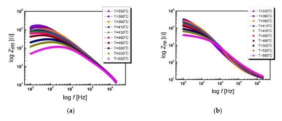
**Figure 5.** Frequency dependence of the impedance of the imaginary part,  $Z_{im}$ , (**a**) and the real part,  $Z_{re}$ , (**b**) on the frequency, *f*, at different temperatures of BLT4 ceramics.
