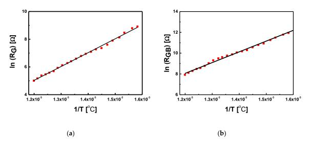
**Figure 11.** Dependence of the natural logarithm of the grain (**a**) and grain boundary (**b**) values calculated on the basis of impedance spectra as a function of temperature inverse of BLT4 ceramics.
