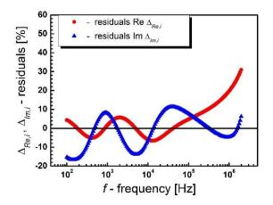
**Figure 8.** Frequency relationship of approximation errors of the real part and the imaginary impedance of BLT 4 ceramics, calculated at T = 377 °C.
