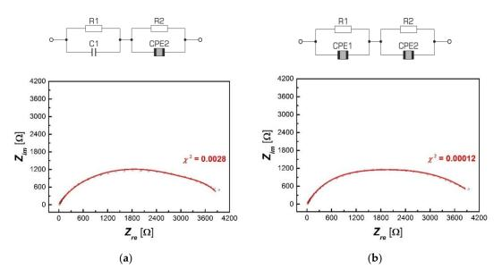
**Figure 10.** Graphs of the dependence of the imaginary part of impedance ( $Z_{im}$ ) on its real part ( $Z_{re}$ ) together with the matching spectrum for selected electric replacement models obtained at T = 455 °C; for a system with a single CPE (**a**) and for a system with a double CPE (**b**).
