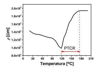
Figure 12. Temperature dependence of resistivity for BLT4 ceramics.
