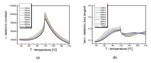
**Figure 3.** Temperature dependence of electric permittivity (**a**) and tangent of the dielectric loss angle (**b**) on the temperature and frequency of the measuring field for BLT4 ceramics.
