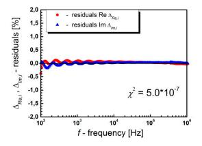
**Figure 6.** Residual spectrum (residuals) showing the frequency relationship of the relative difference between the experimental data and the data obtained as a result of the K-K test at T = 230 °C for BLT4 ceramics.
