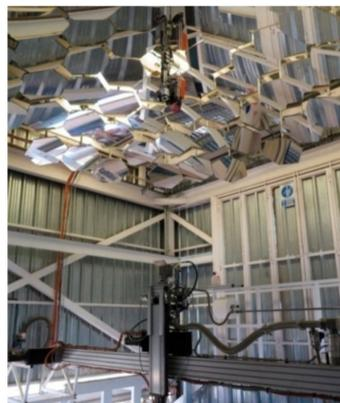
**Figure 1.** SF5 vertical axis solar furnace (test room).
