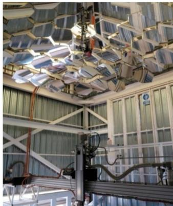
**Figure 1.** SF5 vertical axis solar furnace (test room).
