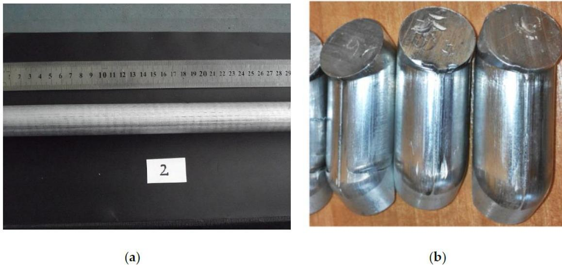
**Figure 1.** AlCu4MgSi alloy (AW 2017A), (a) ingot obtained in horizontal continuous casting, (b) ingot fragments plastically treated by equal channel angular pressing (ECAP).
