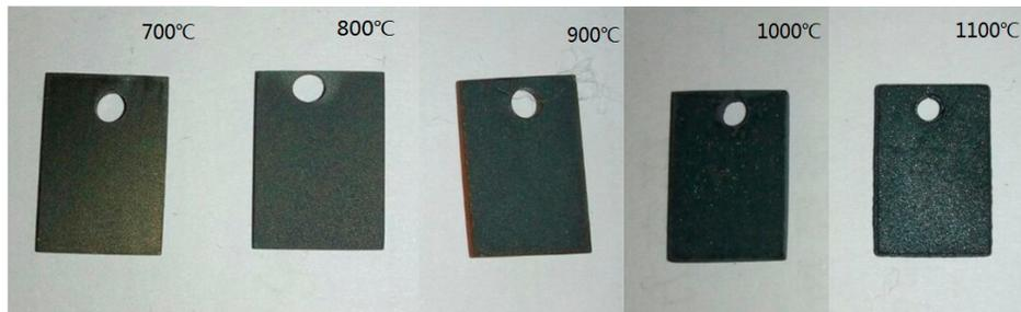
**Figure 2.** Macroscopic morphology of the Fe-1Cr-0.2Si steel specimens observed by the naked eye after 120 min of oxidation.
