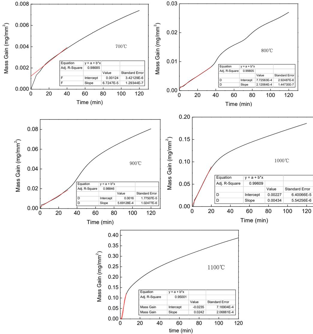
**Figure 13.** The kinetic plots obtained from the oxidation of steel in a short time. (a) 700 °C; (b) 800 °C; (c) 900 °C; (d) 1000 °C; (e) 1100 °C.
