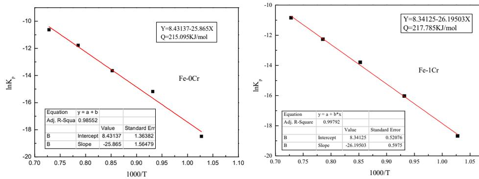
Figure 12. A fitting curve for steel ( $\ln K_p$  vs.  $1000/T$ ). (a) Fe-1Cr; (b) Fe-0Cr.
