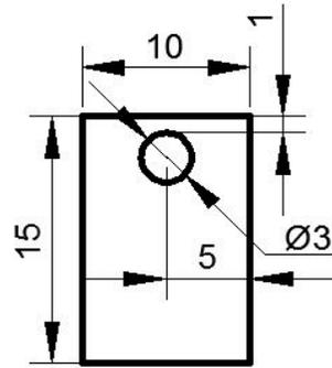
**Figure 1.** The location of the specimen borehole.
