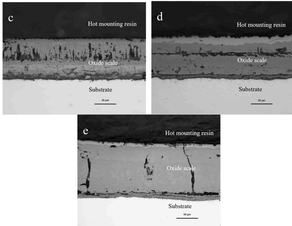
**Figure 5.** Cross-sectional morphology of the specimens observed under the metallurgical microscope. (a) 700 °C; (b) 800 °C; (c) 900 °C; (d) 1000 °C; (e) 1100 °C.
