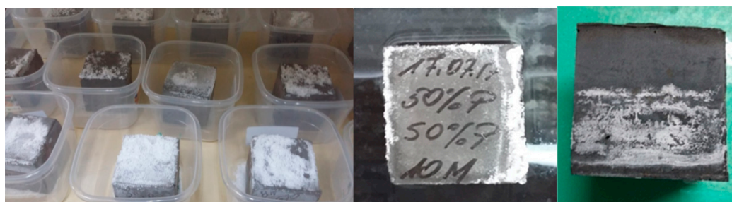
Figure 7. Appearance of selected samples during tests for susceptibility to efflorescence (after 14 days); samples cured at ambient conditions.
