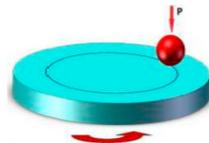
**Figure 1.** Scheme of the ball-on-disc test [7].
