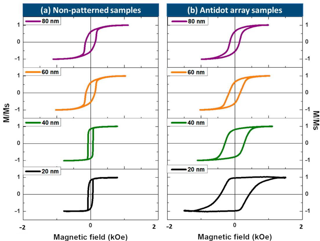
**Figure 3.** Transversal Kerr hysteresis loops for  $\text{Fe}_{70}\text{Pd}_{30}$  with different thicknesses (20, 40, 60 and 80 nm) for (a) non-patterned thin films and (b) antidot array thin films.
