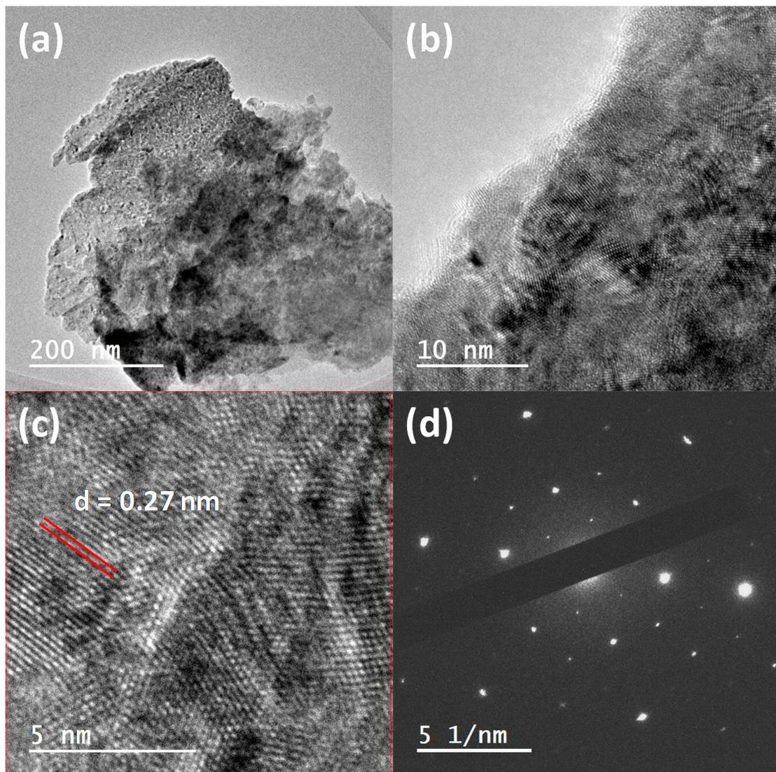
**Figure 2.** (a–c) HR-TEM images of Fe–Pd continuous thin film with a 20 nm layer thickness taken at different magnifications. Regions with different directions of the crystallographic planes are shown in (b,c). (d) The SAED image along a direction near a two-fold symmetry axis (see text).
