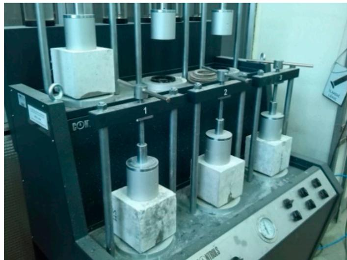
**Figure 7.** Testing of water penetration in cracked specimens.
