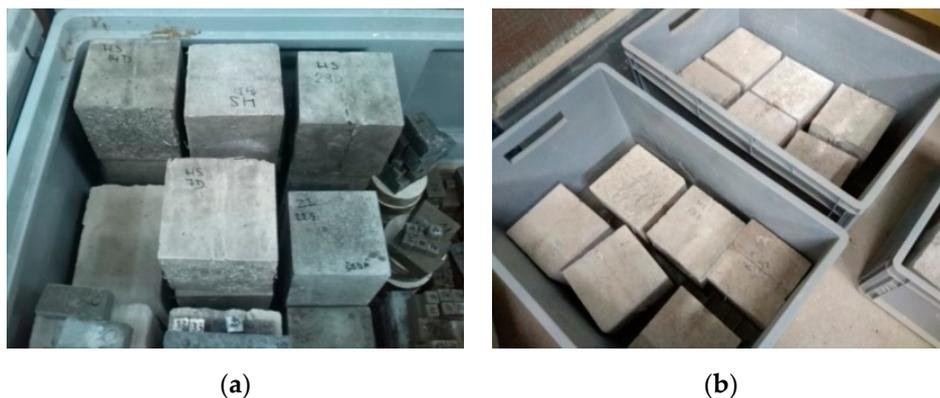
**Figure 2.** Placement of specimens. (a) Specimens in the tank with a humid environment. (b) Specimens in tanks with a water level about 20 mm above the bottom.
