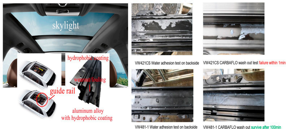
Figure S5. The pictures of the guide rails that crack (general anodizing film) and keep complete (robust superhydrophobic film).
