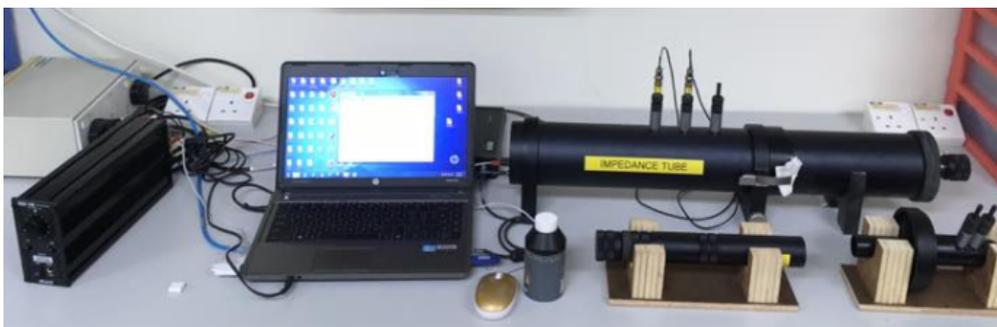
**Figure 4.** Impedance tube instrument.
