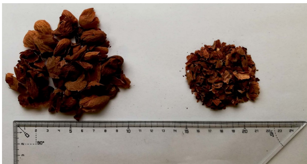
Figure 3. Aggregates used. (On the left) almond residue in its true state used for AS0_GA, (on the right) almond residue in ground state used for AS1_PVA.
