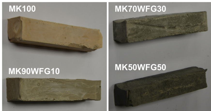
Figure 4. Appearance of the 28-day cured specimens.
