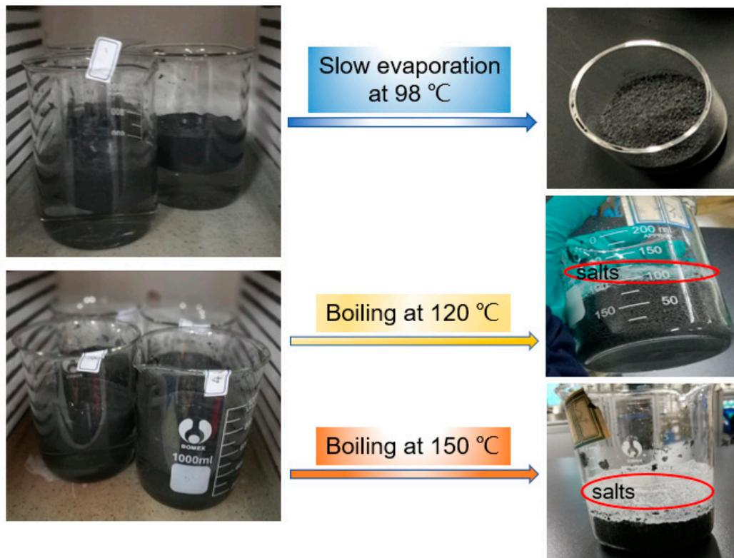
**Figure 6.** Photographs of the  $\text{Ca}(\text{NO}_3)_2\text{-NaNO}_3/\text{EG}$  composite slurries dried at 98, 120, and 150 °C for 5 h.
