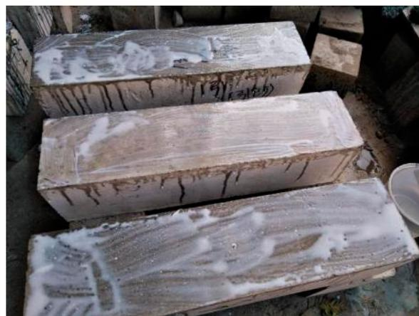
**Figure 1.** Prism concrete specimens applied with a repellent agent of BS4004.
