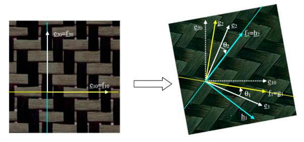
**Figure 1.** Orthogonal frames  $g(\underline{g}_1 = \underline{f}_1, \underline{g}_2)$  and  $h(\underline{h}_1, \underline{h}_2 = \underline{f}_2)$  defined from the direction of the warp and weft yarns.
