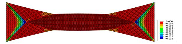
Figure 7. Inelastic shear strain of a specimen obtained via bias extension test after loading in tension.
