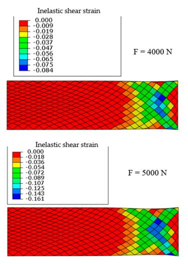
Figure 10. Inelastic shear strain for 4000 and 5000 N.
