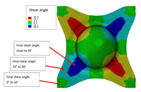
Figure 4. Shear angles after a hemispherical forming.
