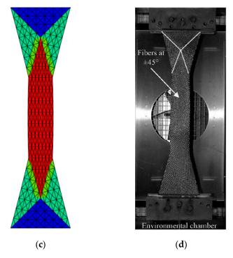
**Figure 2.** Bias extension test. (a) initial position; (b) development of sheared zone (C), half-sheared zone (B) and non-sheared zone (A); (c) finite element simulation and experimental thermoforming; (d) experiments.
