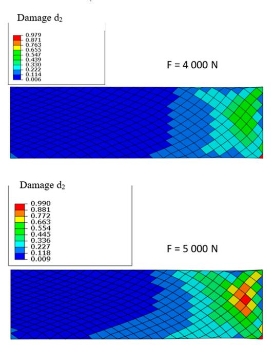
**Figure 9.** Matrix damage  $d_2$  for for 4000 and 5000 N.
