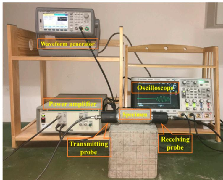
Figure 4. Ultrasonic testing setup.
