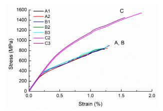
**Figure 5.** Stress–strain curves of SLM AISI 420 built in three directions. (A, B, and C denote the specimens built along the thickness, width, and length directions, respectively, as shown in Figure 2. A1, A2, and others individually represent each specimen ID number).
