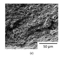
**Figure 7.** SEM micrographs of a Group B specimen: (**a**) Overview of fracture surface; (**b**) high-magnification view of the outlined fracture origin zone in (**a**); (**c**) high-magnification view of a region away from the fracture origin.
