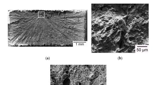
**Figure 8.** SEM micrographs of a Group C specimen: (**a**) Overview of fracture surface; (**b**) high-magnification view of the outlined fracture origin zone in (**a**); (**c**) high-magnification view of a region away from the fracture origin.
