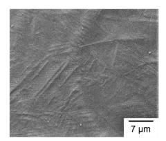
Figure 13. SEM micrograph of needle-like martensite laths at the top surface of as-built SLM 420 sample.
