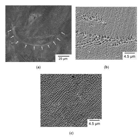
**Figure 12.** Representative SEM micrographs of melt pool: (a) Low-magnification view of vertical cross-section; (b) high-magnification view of melt pool boundary in vertical cross-section; (c) high-magnification view of melt pool center in horizontal cross-section.
