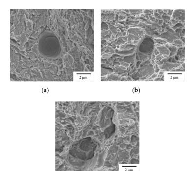
**Figure 9.** SEM micrographs of micro-pores and cleavage facets observed on the fracture surface: (a) Group A; (b) Group B; (c) Group C.
