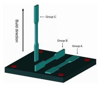
Figure 2. Schematic of build direction for each group of specimen.
