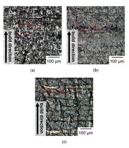
**Figure 11.** Optical microscopy (OM) micrographs of representative microstructure in the SLM specimens: (a) Group A; (b) Group B; (c) Group C. (Arrow indicates the build direction.).
