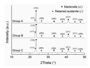
Figure 10. XRD results of SLM AISI 420 specimens built in various directions.Table 4. Phase content in SLM AISI 420 specimens with various build directions.
