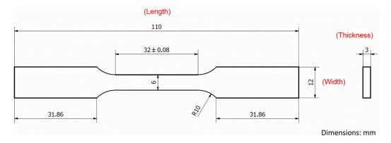
Figure 1. Geometry and dimensions of tensile specimen.
