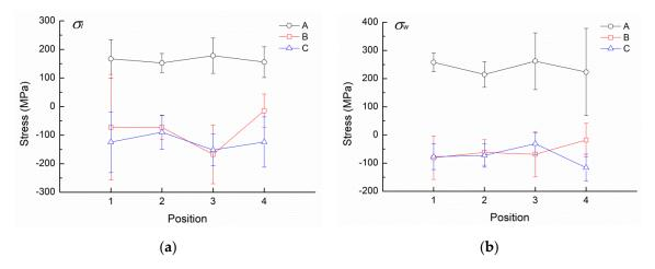
**Figure 4.** Results of residual stress measurement: (a)  $\sigma_l$ ; (b)  $\sigma_w$ . (A, B, and C denote the specimens built along the thickness, width, and length directions, respectively, as shown in Figure 2).
