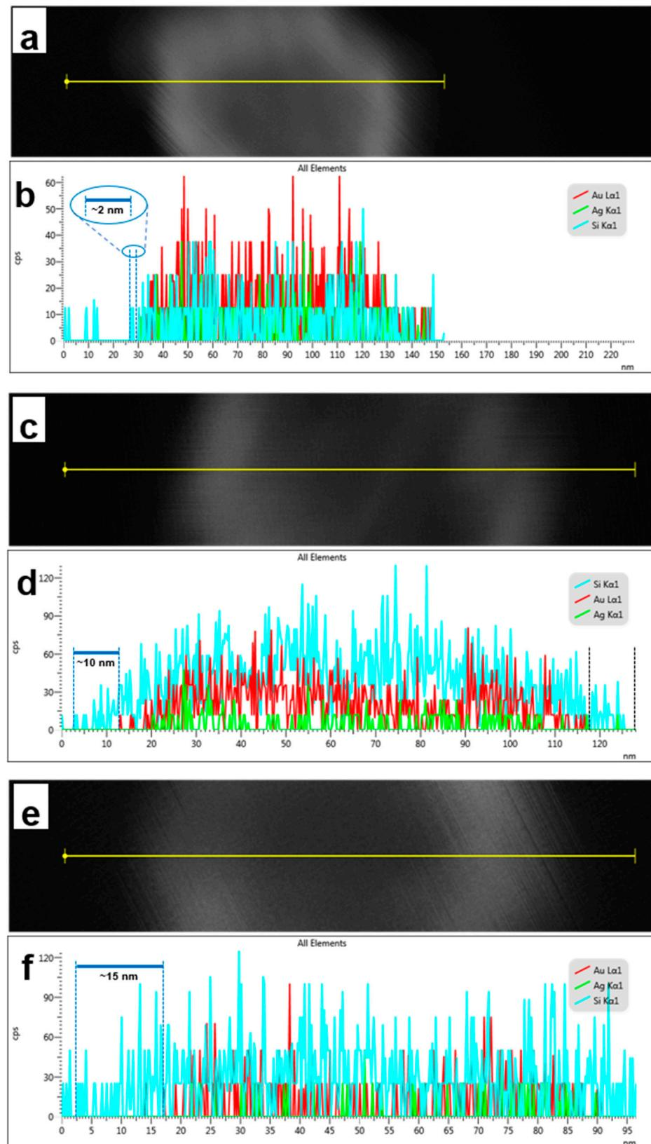
**Figure S2.** STEM images and corresponding energy-dispersive X-ray (EDX) line scan spectra of  $\text{SiO}_2$ -coated gold-silver nanoshells with (a,b) 2 nm, (c,d) 10 nm, and (e,f) 15 nm silica shell.
