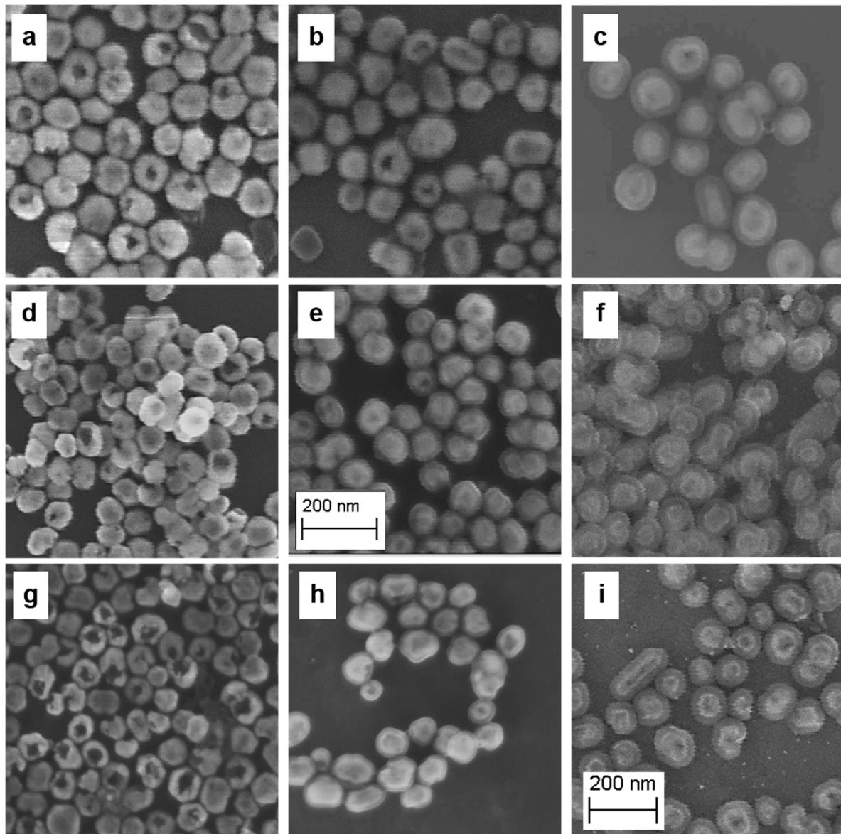
**Figure S1.** SEM images of silica-coated gold-silver nanoshells with the indicated LSPR peak positions. (a–c) GS-NS (500), (d–f) GS-NS (700), and (g–i) GS-NS (900) with ~2 nm, ~10 nm, and ~15 nm, respectively. LSPR = localized surface plasmon resonance
