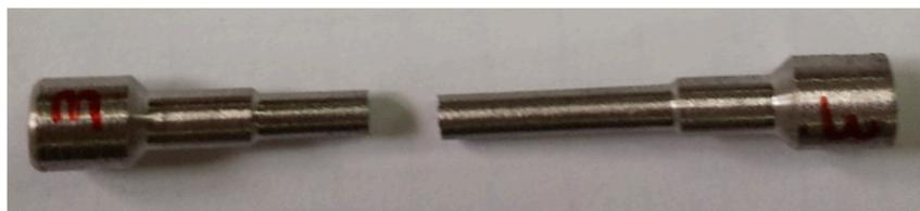
**Figure 10.** Sample THA-1 with THA-3 fractured in the zone distant from the joint line material THA-3.
