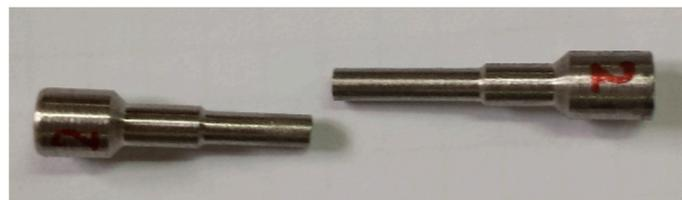
**Figure 9.** Sample THA-2 with THA-3 fractured in the joint line or in its immediate vicinity.
