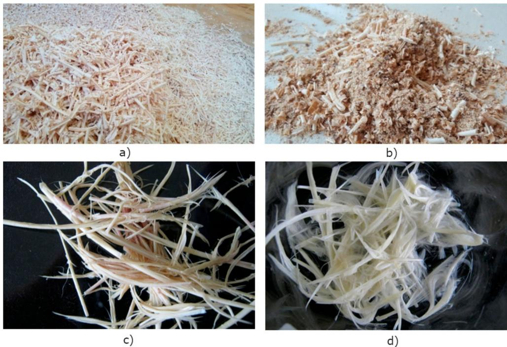
**Figure 1.** Waste residues: (a) wood shavings; (b) mixed wood residues; (c) waste poultry feathers after industrial precleaning; and (d) feathers after the laboratory washing and rinsing process.
