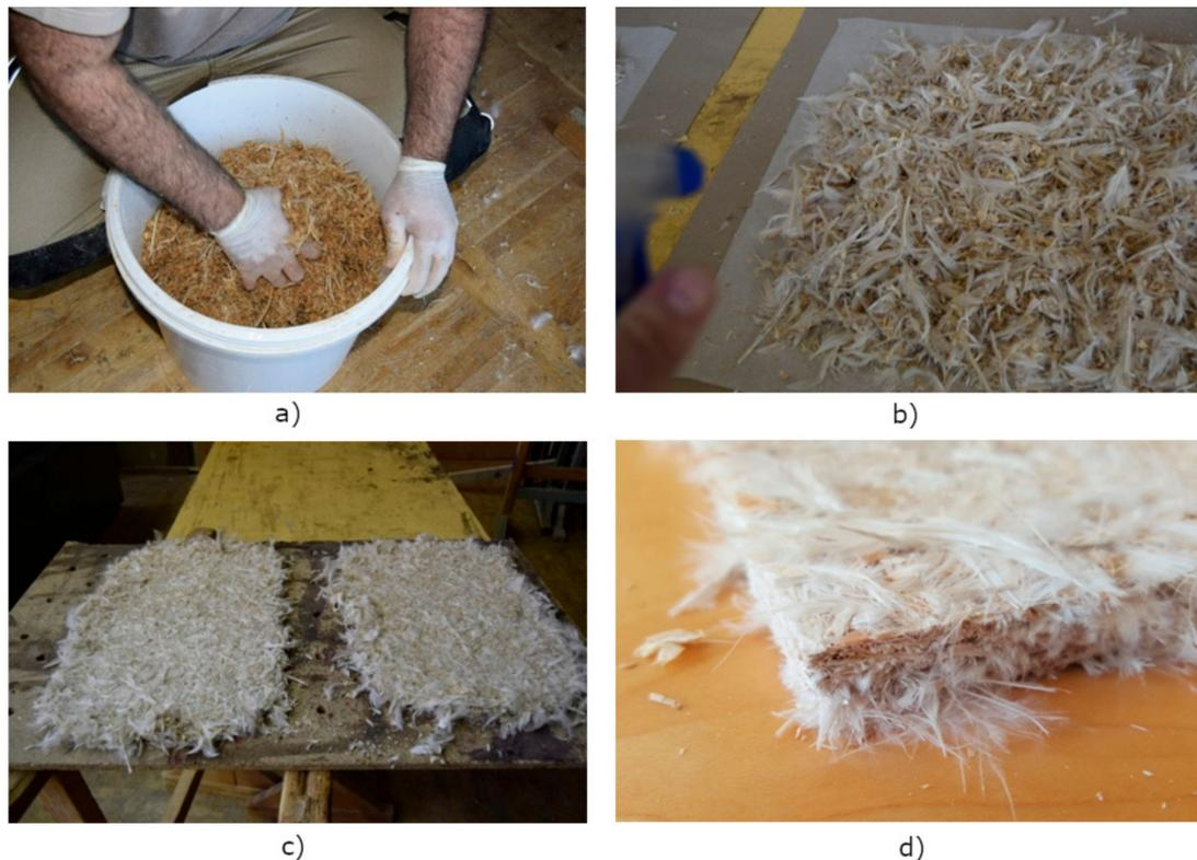
**Figure 4.** Preparation of fibreboards: (a) wood mixture; (b) mixture of feathers and wood shavings; (c) fibreboard samples after pressing; and (d) cut out fibreboards for testing.
