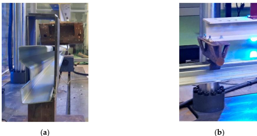
Figure 4. Details of the laboratory stand: (a) beam support detail; (b) of the load application through the hot-rolled C100 profile.
