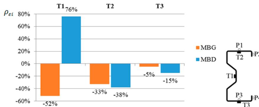
Figure 8. Strain percentage change in relation to the beams without reinforcement, read from a strain gauge at a load level of 25 kN and for different locations of the CFRP tape.
