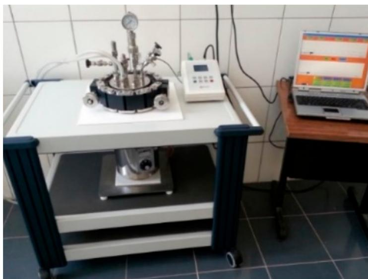
**Figure 1.** The Berghof autoclave experimental device.
