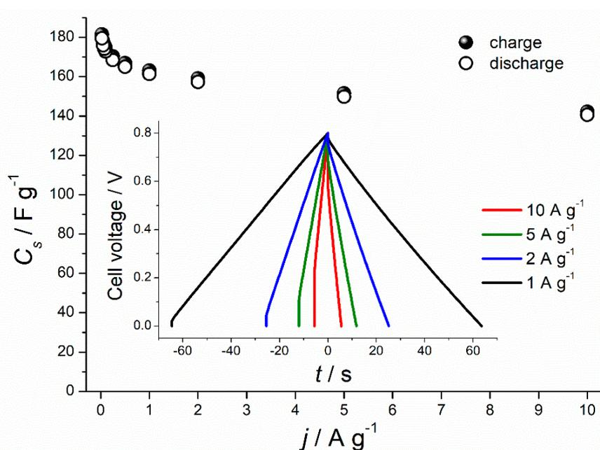
**Figure 5.** Specific capacitance values recorded for C-KOH sample at different current densities. Inset: galvanostatic charge-discharge (GCD) profiles at high current densities ( $1\text{--}10 \text{ A g}^{-1}$ ).
