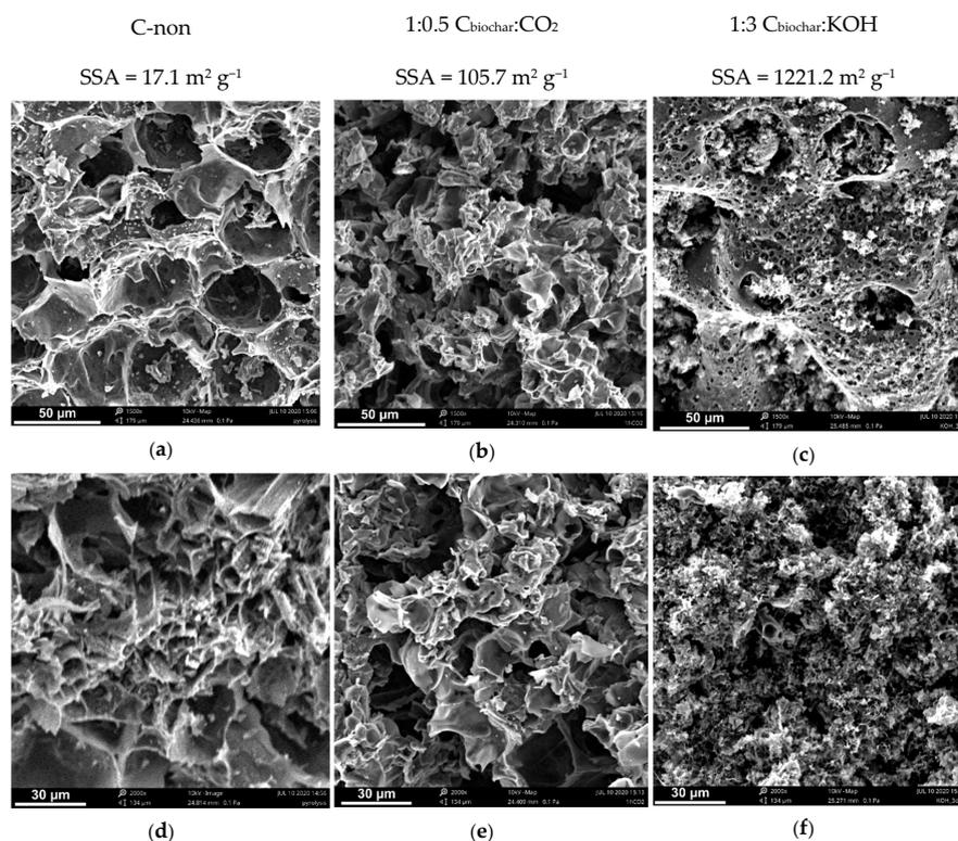
**Figure 2.** SEM images of: raw biochar (a,d); biochar after physical activation (b,e); biochar after chemical activation (c,f).
