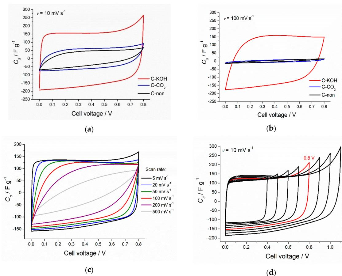
**Figure 3.** CV curves of the chestnut-derived activated carbons recorded at  $10 \text{ mV s}^{-1}$  (a), and at  $100 \text{ mV s}^{-1}$  (b). CV curve for chemically activated carbon (3:1 by weight with KOH) recorded at different scan rates (c), and for various potential windows (d), CV at 0.8 V (marked red) was selected for further experiments in the two-electrode setup.
