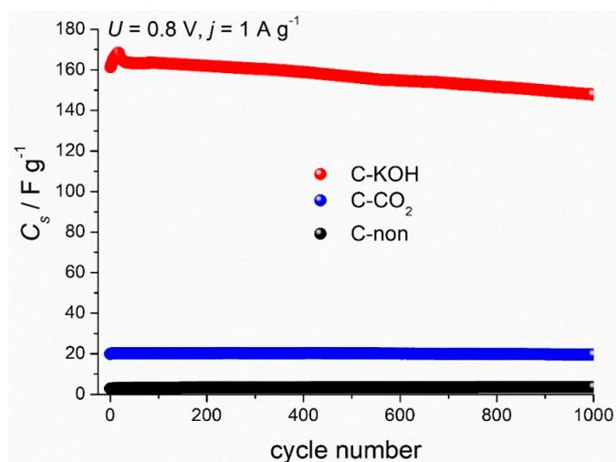
**Figure 7.** Electrochemical performance of C-KOH activated carbons; 6 M KOH electrolyte; GCD measured at 1 A g<sup>-1</sup> and 0.8 V cell voltage.
