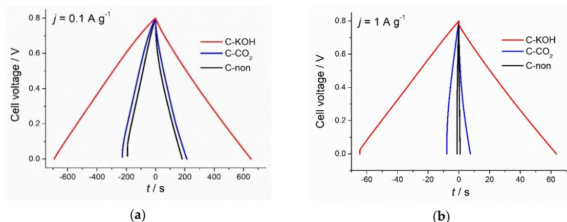
**Figure 4.** Charge-discharge profiles of C-KOH, C-CO<sub>2</sub> and C-non samples at  $0.1 \text{ A g}^{-1}$  (a) and  $1 \text{ A g}^{-1}$  (b).
