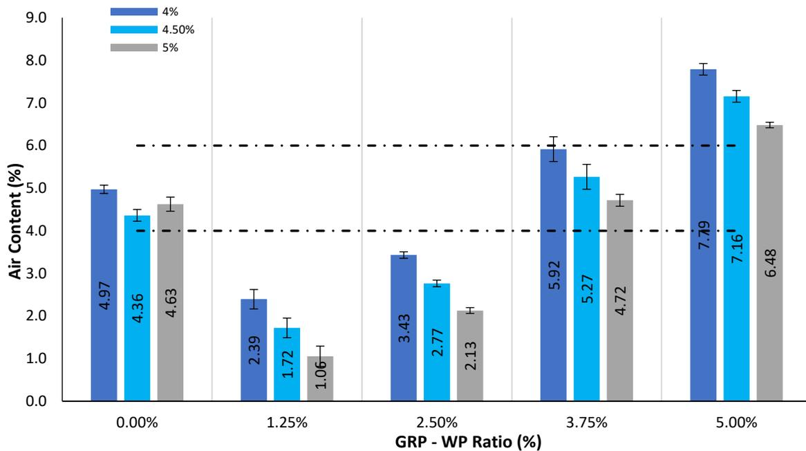
Figure 8. Comparison of air content (Va) results for the 45 samples tested.
