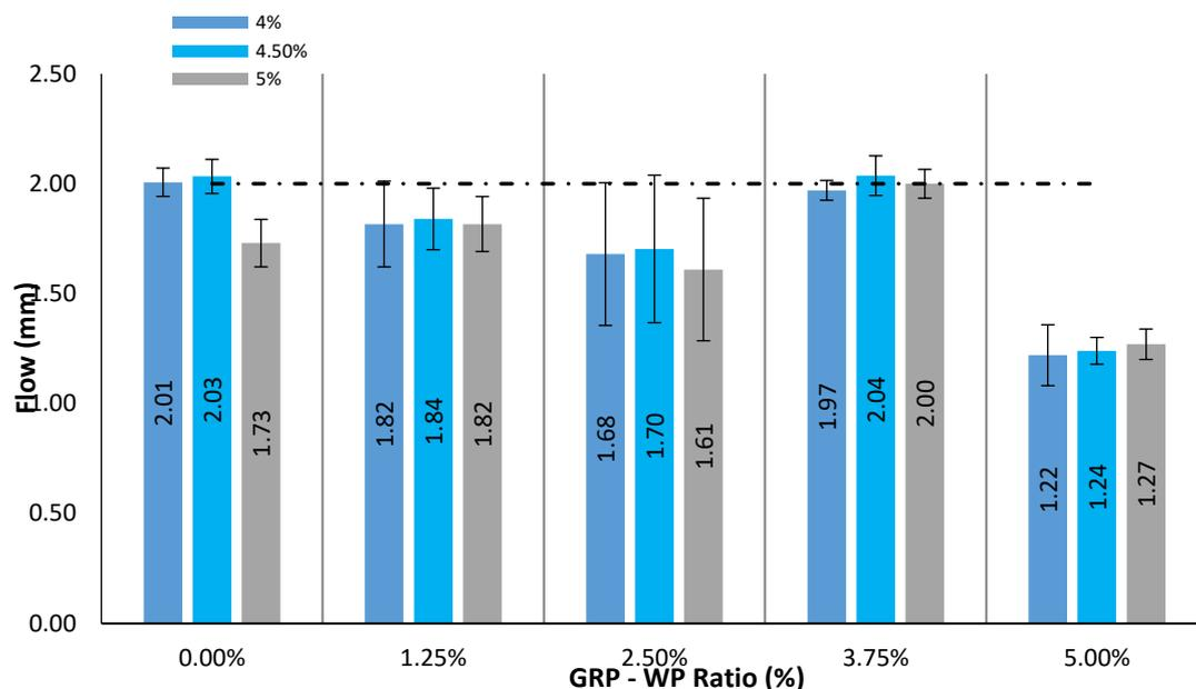
Figure 5. Comparison of flow results for the 45 samples tested.
