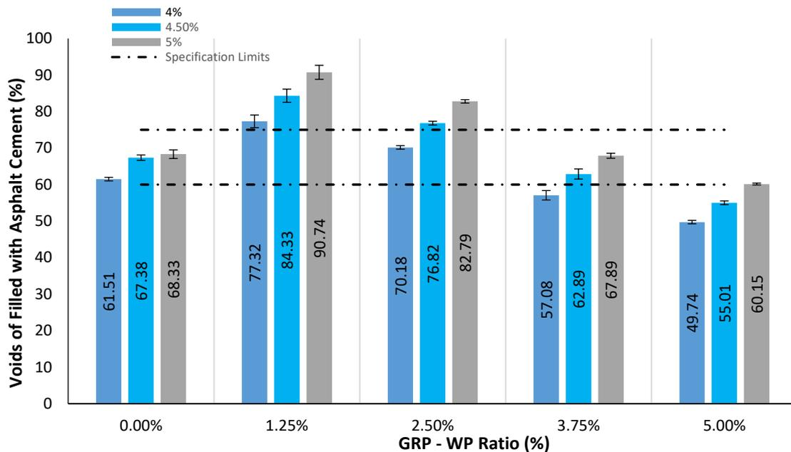
Figure 7. Comparison of VFA results for the 45 samples tested.
