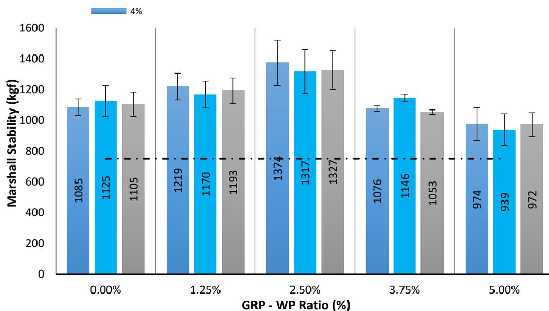
**Figure 4.** Comparison of MS results for the 45 samples tested.
