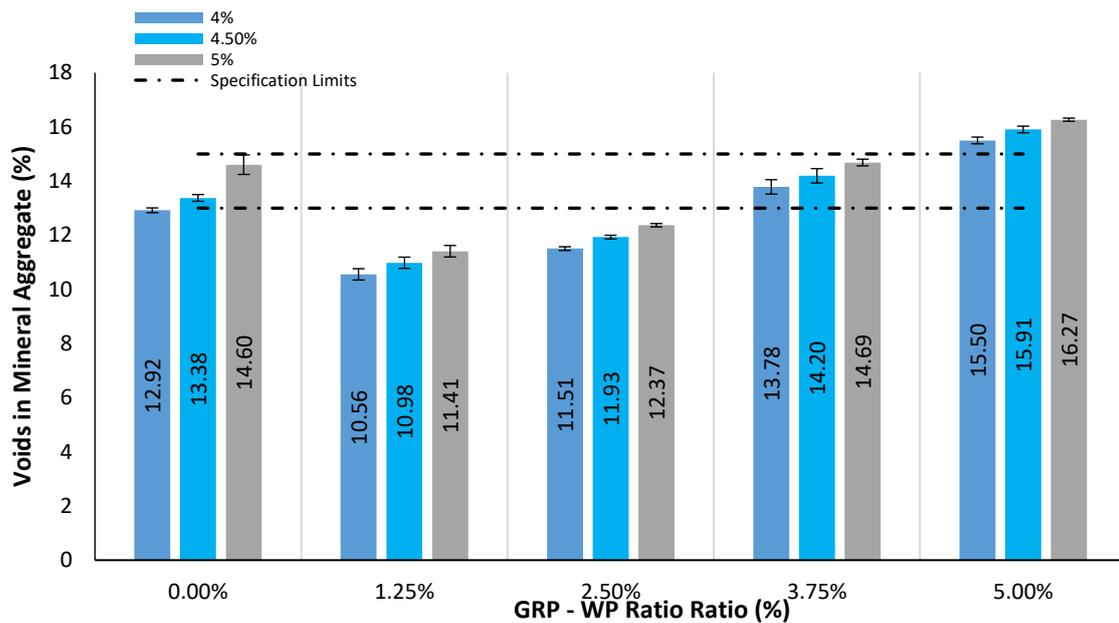
Figure 6. Comparison of VMA results for the 45 samples tested.
