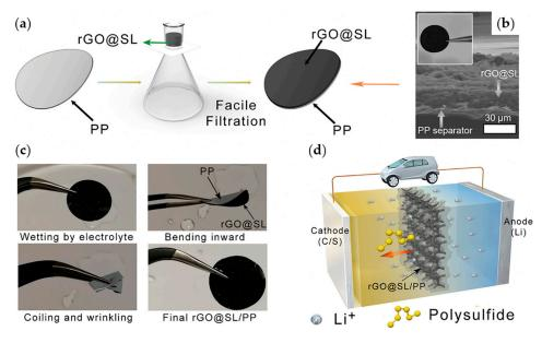
**Figure 12.** (a) Schematic of the fabrication procedure of the rGO@SL/PP separator (b) SEM image of the rGO@SL/PP separator (c) Digital photos of the rGO@SL/PP separator under various mechanical stresses. (d) Schematic of the rGO@SL/PP separators inhibiting shuttle effects in LSBs. Reprinted with permission from [141]. Copyright (2018) Elsevier Inc.
