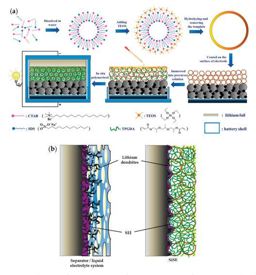
**Figure 16.** (a) Illustration for preparation steps of SiSE. (b) Comparison of SiSE to separator/liquid electrolyte system. Reprinted with permission from [161]. Copyright (2016) John Wiley and Sons.
