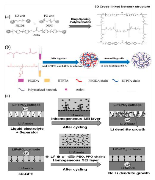
**Figure 17.** (a) Illustration of the synthesis of the GPE. Reprinted with permission from [148]. Copyright (2017) John Wiley and Sons. (b) Step process for in situ polymerization of GPE. Reprinted with permission from [162]. Copyright (2018) John Wiley and Sons. (c) Schematics of the changes in the Li electrodes using a liquid electrolyte and 3D-GPE during the Li plating/stripping. Reprinted with permission from [148]. Copyright (2017) John Wiley and Sons.
