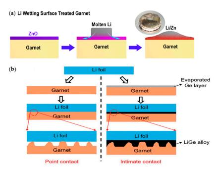
**Figure 14.** (a) ZnO-coated garnet electrolyte. Reprinted with permission from [153]. Copyright (2017) American Chemical Society.; (b) Ge-coated garnet electrolyte. Reprinted with permission from [154]. Copyright (2017) John Wiley and Sons.
