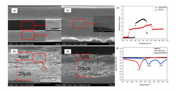
**Figure 2.** (**a**–**d**) SEM images: (**a**,**c**) cross-section of a PP/PE/PP separator before and after hot treatment at 140 °C for 0.5 h; (**b**,**d**) cross-section of a PE-PI-S nonwoven membrane before and after hot treatment 140 °C for 0.5 h. (**e**) Impedance change with a heating rate 1 °C min<sup>-1</sup> of the PP/PE/PP separator and PE-PI-S nonwoven membrane. (**f**) differential scanning calorimetry of the PI, PP/PE/PP, and PE/PI/S membranes [48]. Copyright (2015) Elsevier B.V.
