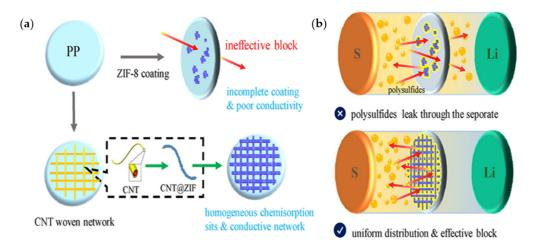
**Figure 13.** (a) Schematics of ZIF-8 and the CNT@ZIF composite modified separators (b) Li-S battery configuration with the modified separators. Reprinted with permission from [142]. Copyright (2018) Elsevier B.V.
