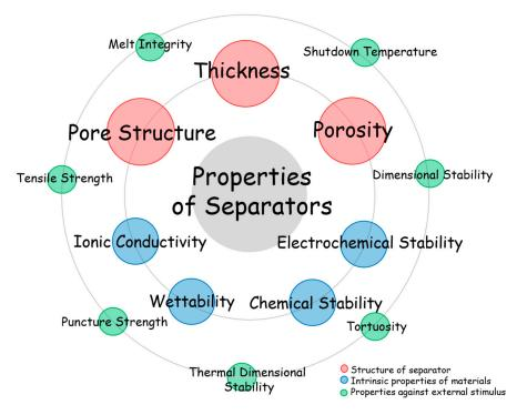
Figure 1. Illustration of the key properties of separators.
