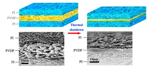
**Figure 8.** Figure and cross-sectional SEM images of the PI/PVDF/PI membrane before and after the hot melting and shutdown behavior of the PVDF nanofibers layer. Reprinted with permission from [115]. Copyright (2015) Elsevier Ltd.
