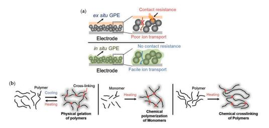
**Figure 18.** (**a**) Ex-situ GPE and in situ GPE. (**b**) Gelation via cross-linking of polymers. Reprinted with permission from [164]. Copyright (2018) John Wiley and Sons.
