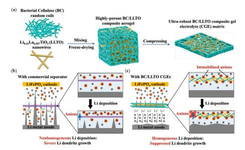
**Figure 19.** Preparation of BC/LLTO CGEs. (**a**) Schematic of the effect of (**b**) a commercial separator and (**c**) a BC/LLTO CGE on Li deposition in a battery. Reprinted with permission from [165]. Copyright (2019) WILEY-VCH.
