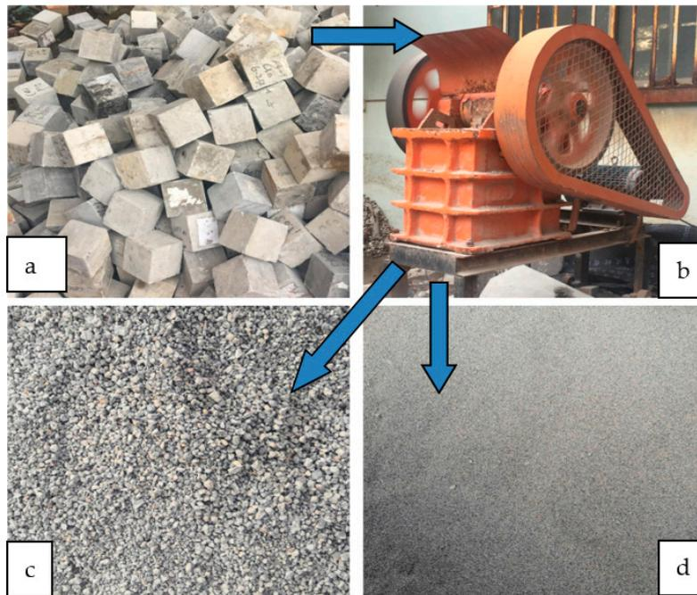
Figure 1. Preparation of recycled aggregate.
