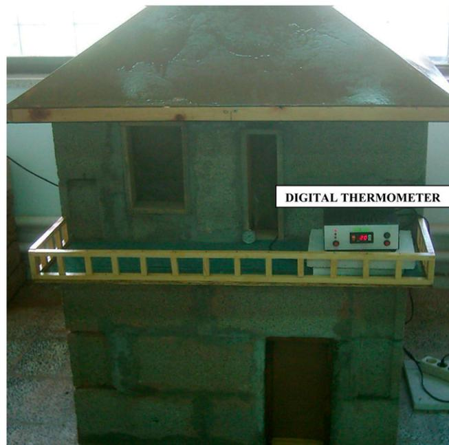
**Figure 14.** Model house built with fiber-reinforced mud bricks [57].
