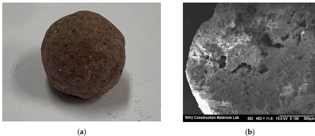
Figure 1. Artificial lightweight aggregate sample: (a) Shape, (b) SEM image.
