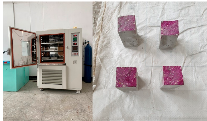
Figure 3. Accelerated-carbonation chamber and samples.
