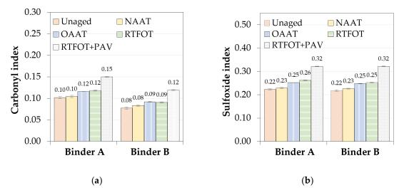
Figure 9. Aging indices: (a) carbonyl and (b) sulfoxides.
