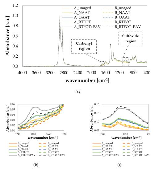
Figure 8. FTIR spectra: (a) complete spectra, (b) carbonyl region, and (c) sulfoxide region.
