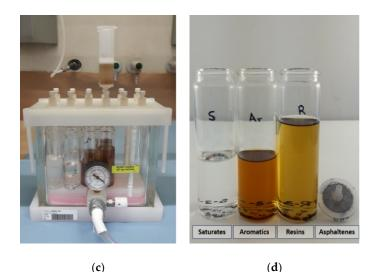
**Figure 2.** Saturates, Aromatics, Resins, and Asphaltenes (SARA) fractionation: (**a**) asphalt binder dissolution, (**b**) filtration of the solution, (**c**) maltene fractionation, and (**d**) SARA fractions.
