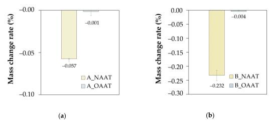
Figure 4. Mass change rate (after NAAT and OAAT aging procedure): (a) binder A; (b) binder B.
