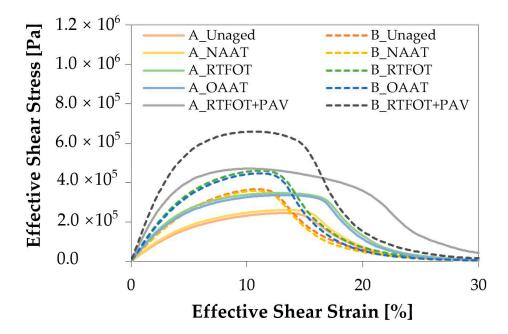
Figure 6. Shear stress (Pa) versus shear strain (%).
