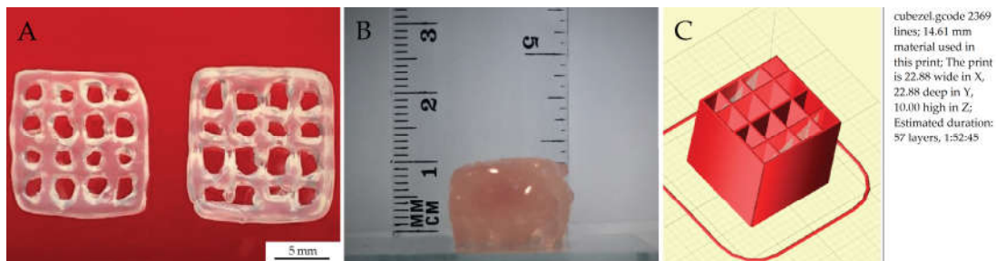
Figure 11. (A) Top view of grids printed on peristaltic based extruder machine, used for printout accuracy tests, (B) height of the printed model obtained from 57 layers, (C) model of the printout with the indicated number of layers.
